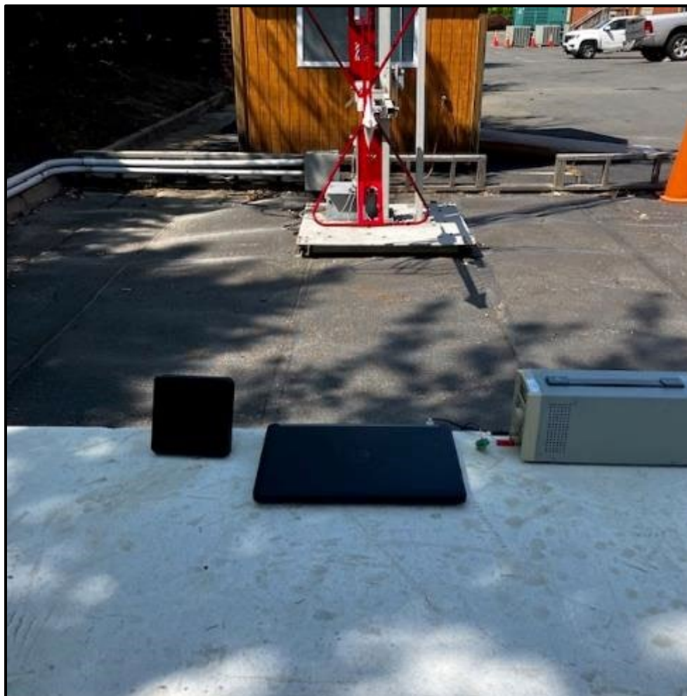
Photograph 1: Radiated Emissions – Front (Less than 1 GHz)
