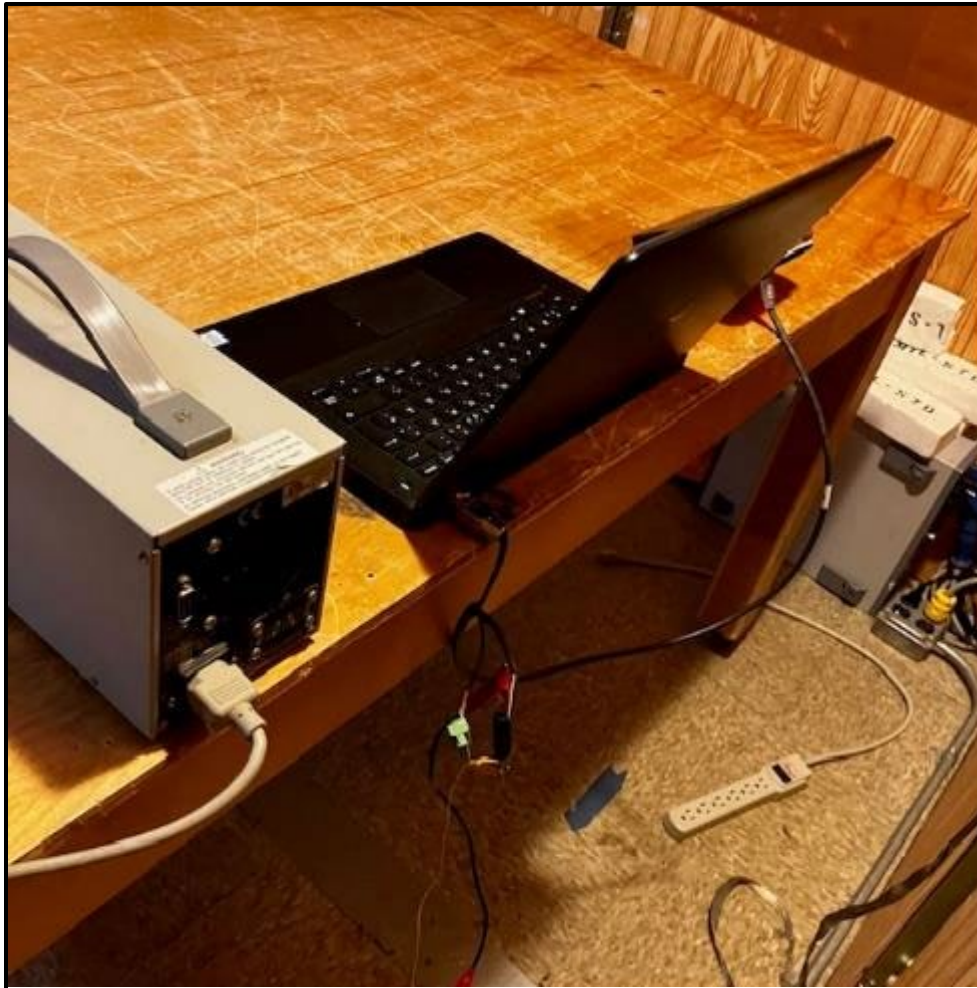
Photograph 7: Conducted Emissions (Back)
