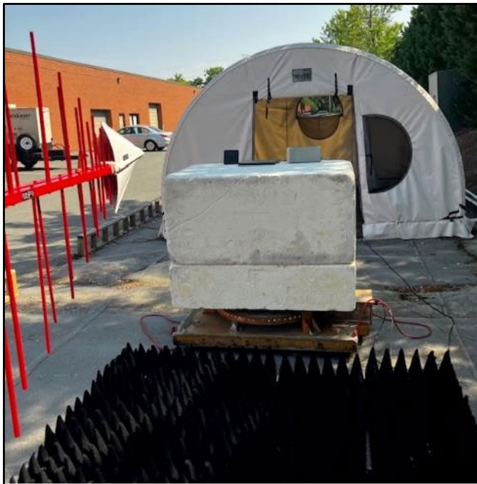
Photograph 3: Radiated Emissions – Front (Greater than 1 GHz)
