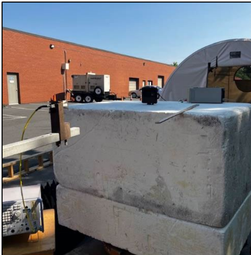
Photograph 5: Radiated Emissions – Front (Greater than 1 GHz) Radar Measurements
