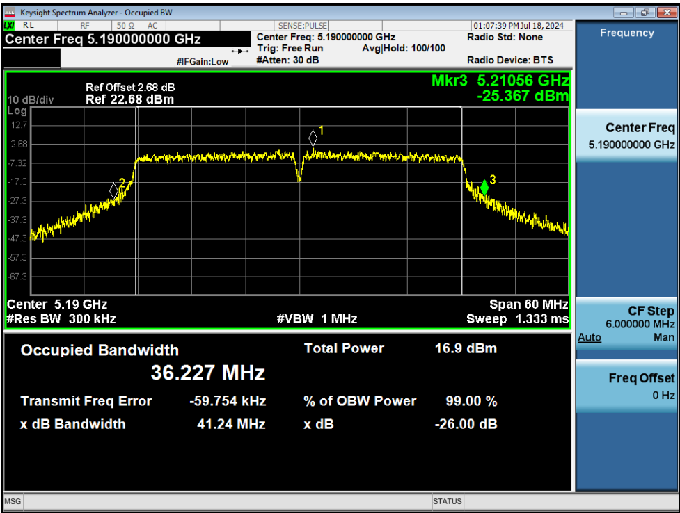
-26dB Bandwidth NVNT ac40 5190MHz Ant1
