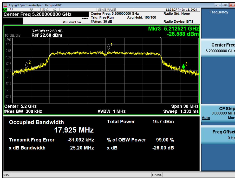
-26dB Bandwidth NVNT n20 5200MHz Ant1
