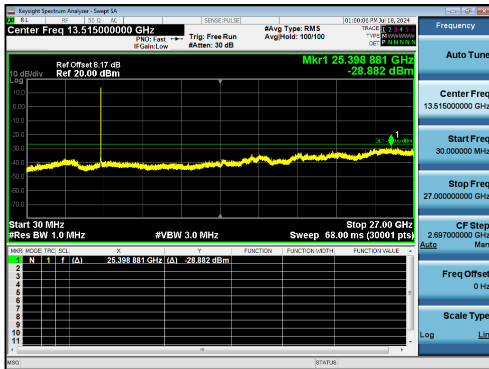
Tx. Spurious NVNT ac20 5200MHz Ant1 Emission
