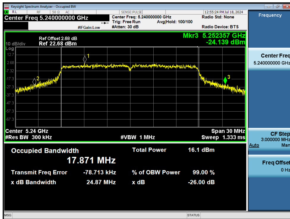
-26dB Bandwidth NVNT n20 5240MHz Ant1
