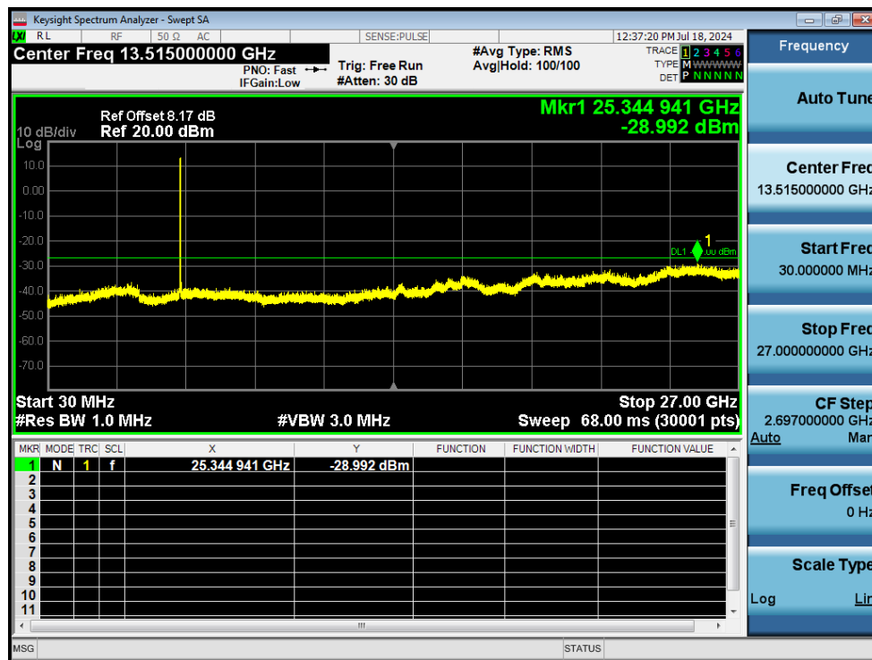
Tx. Spurious NVNT a 5200MHz Ant1 Emission
