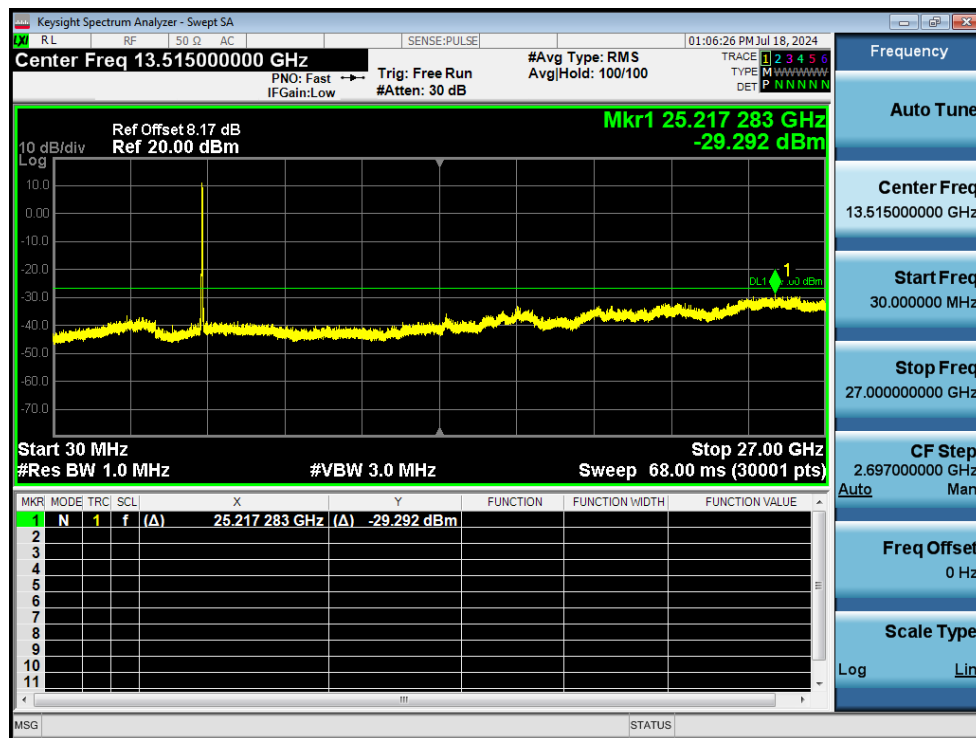
Tx. Spurious NVNT n40 5230MHz Ant1 Emission
