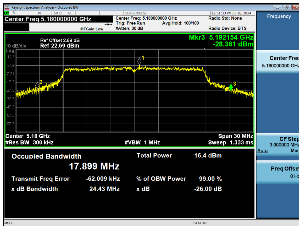
-26dB Bandwidth NVNT n20 5180MHz Ant1
