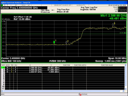
Out Of Band Emission(Left) 8DPSK_3-DH5_Channel Hopping
