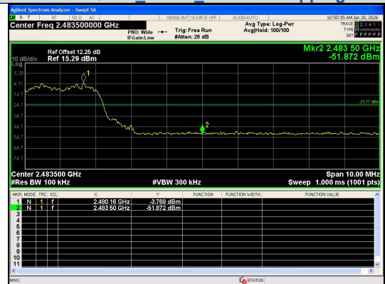
Out Of Band Emission(Right) \pi/4 DQPSK_2-DH5_Channel Hopping
