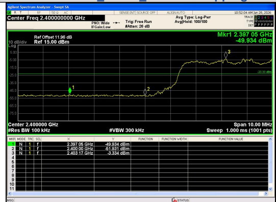
Out Of Band Emission(Left) \pi/4 DQPSK_2-DH5_Channel Hopping
