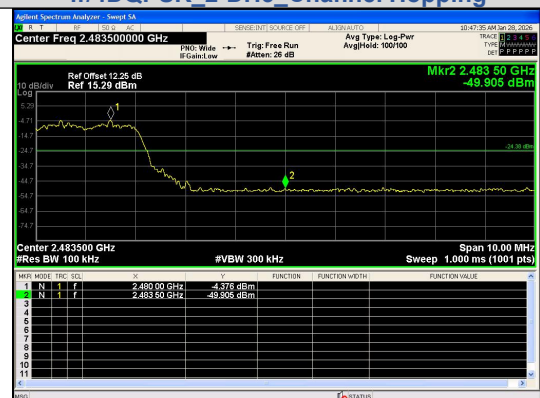
Out Of Band Emission(Right) \pi/4 DQPSK_2-DH5_Channel Hopping
