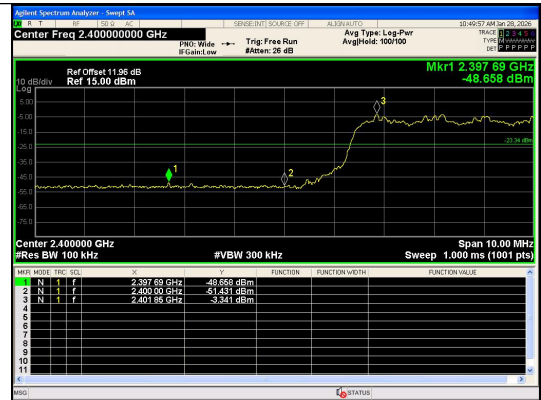
Out Of Band Emission(Left) \pi/4 DQPSK_2-DH5_Channel Hopping
