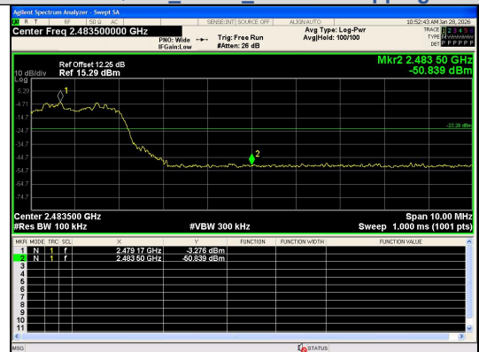
Out Of Band Emission(Right) \pi/4 DQPSK_2-DH5_Channel Hopping
