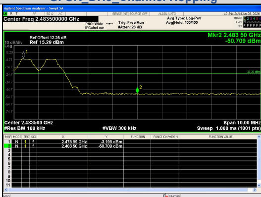
Out Of Band Emission(Right) GFSK_DH5_Channel Hopping
