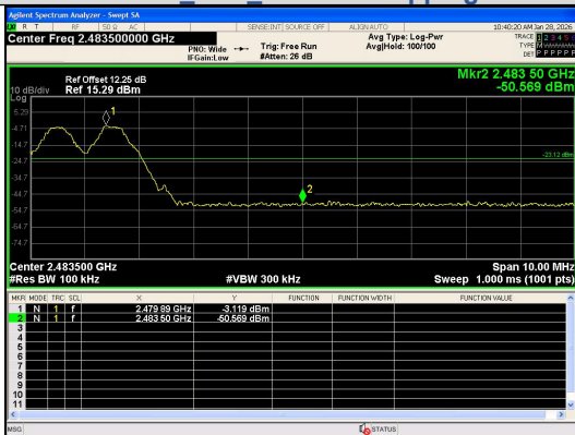
Out Of Band Emission(Right) GFSK_DH5_Channel Hopping
