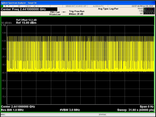
Number of Pulses in 31.6 seconds 8DPSK_3-DH1
