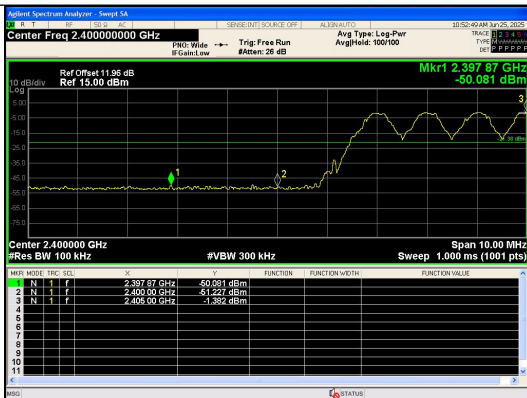
Out Of Band Emission(Left) GFSK_DH5_Channel Hopping
