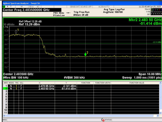
Out Of Band Emission(Right) 8DPSK_3-DH5_Channel Hopping
