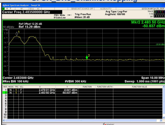
Out Of Band Emission(Right) GFSK_DH5_Channel Hopping
