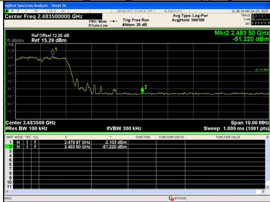
Out Of Band Emission(Right) 8DPSK_3-DH5_Channel Hopping
