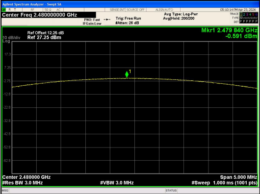
Peak Output Power 8DPSK_Channel 78
