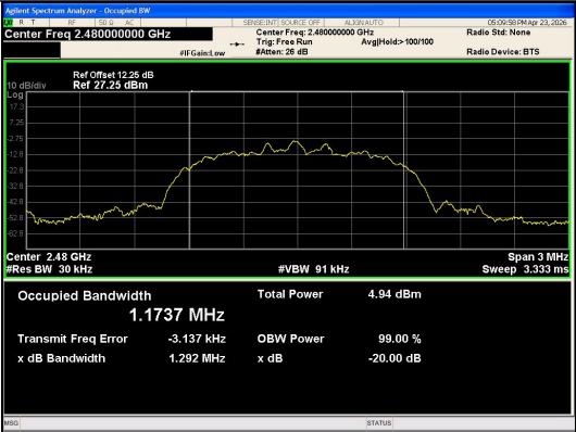
8DPSK 3-DH5 Channel 78
