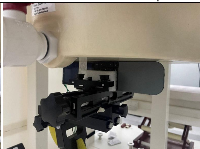
Right Side of EUT with 0 cm Gap
