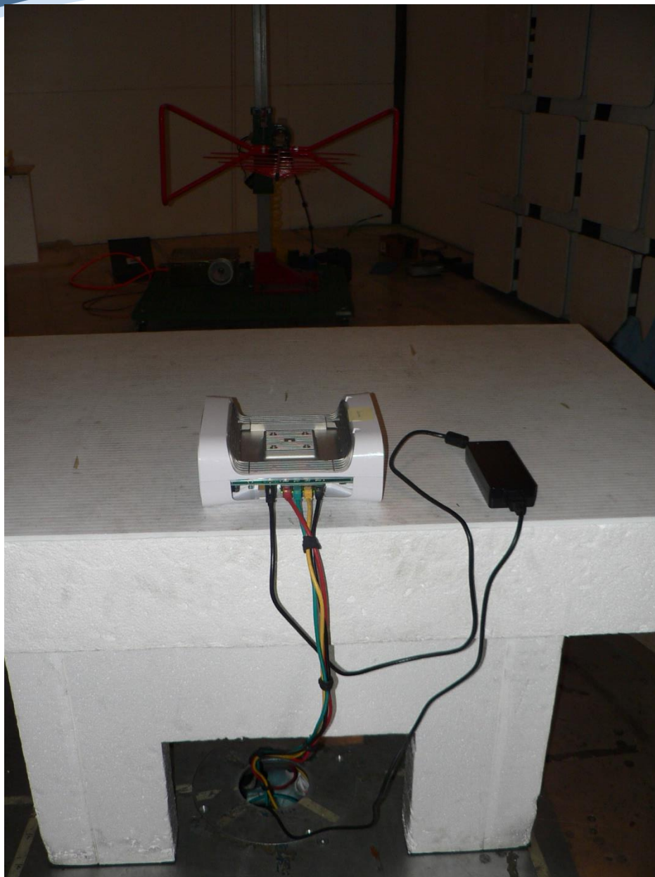
AIRI02 Radiated Emissions 30-1000MHz Back
