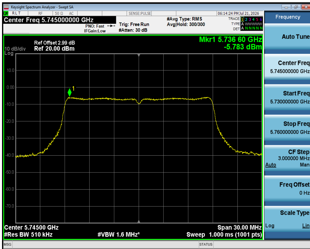
PSD NVNT ac20 5745MHz Ant1
