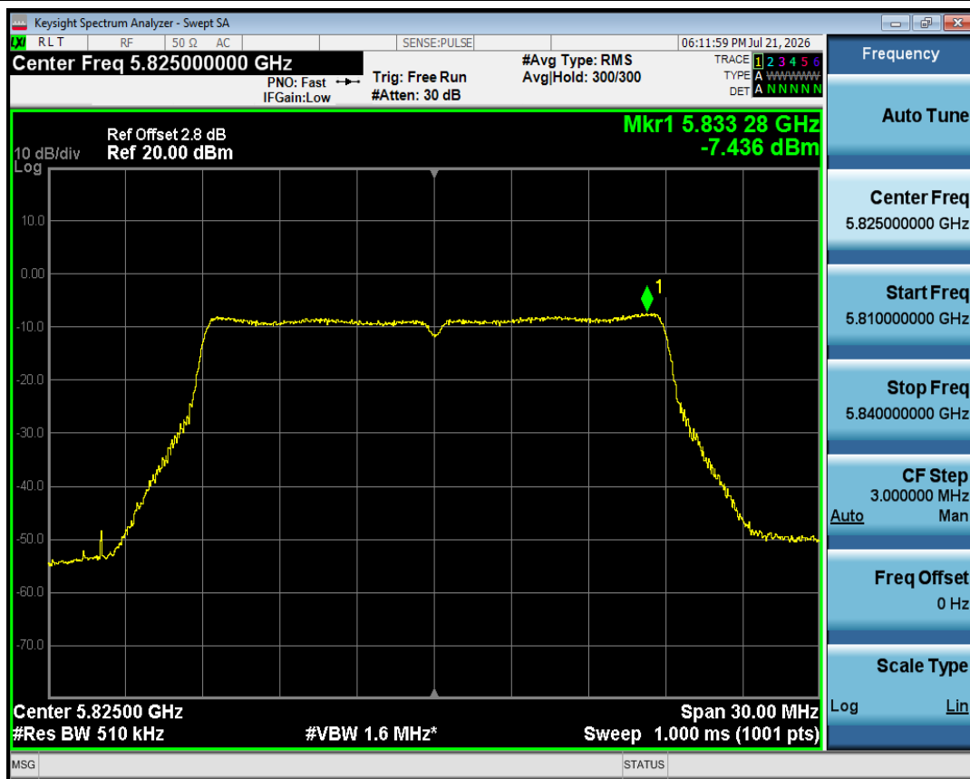
PSD NVNT n20 5825MHz Ant1
