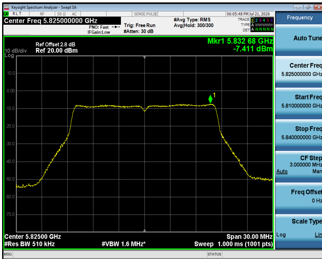
PSD NVNT a 5825MHz Ant1
