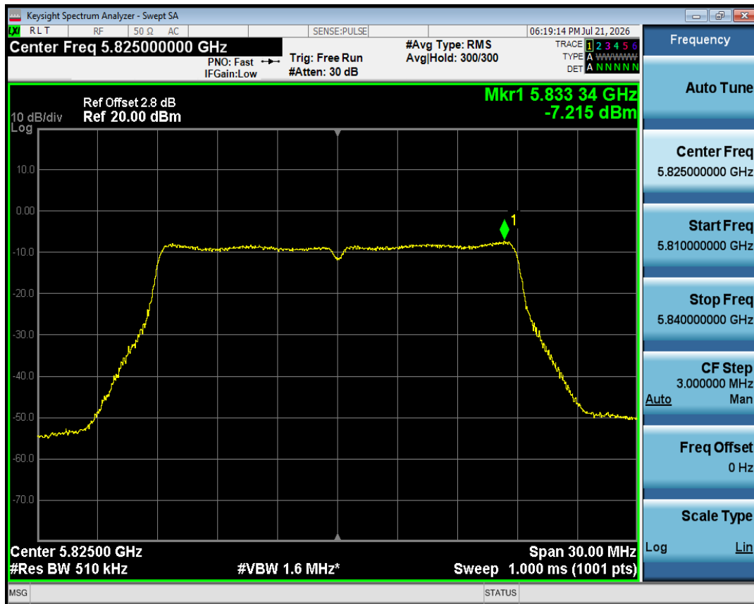
PSD NVNT ac20 5825MHz Ant1
