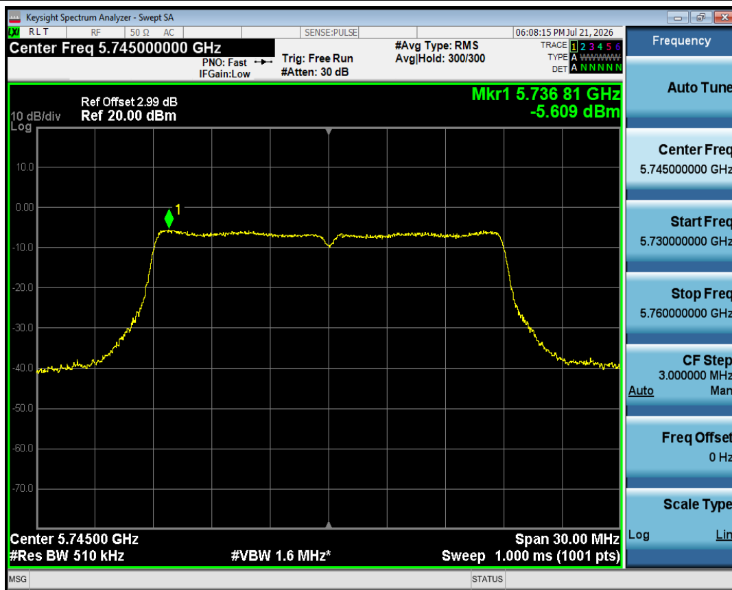
PSD NVNT n20 5745MHz Ant1
