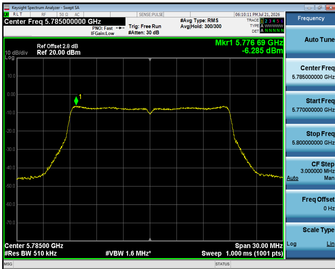
PSD NVNT n20 5785MHz Ant1
