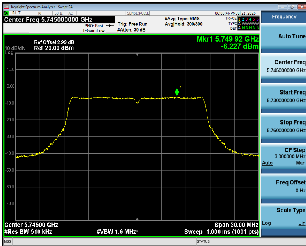
PSD NVNT a 5745MHz Ant1
