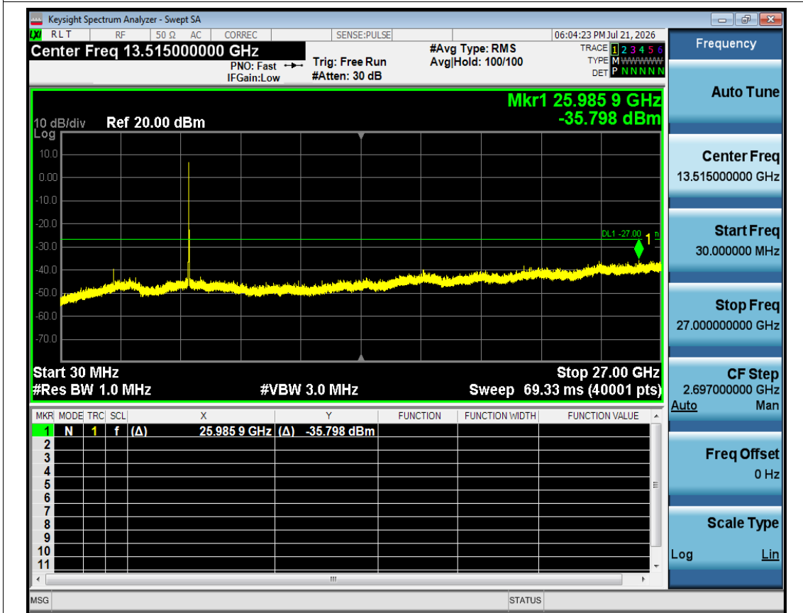
Tx. Spurious NVNT a 5785MHz Ant1 Emission
