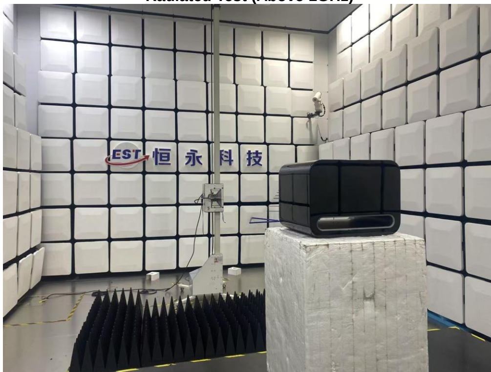
Radiated Test (Above 1GHz)
