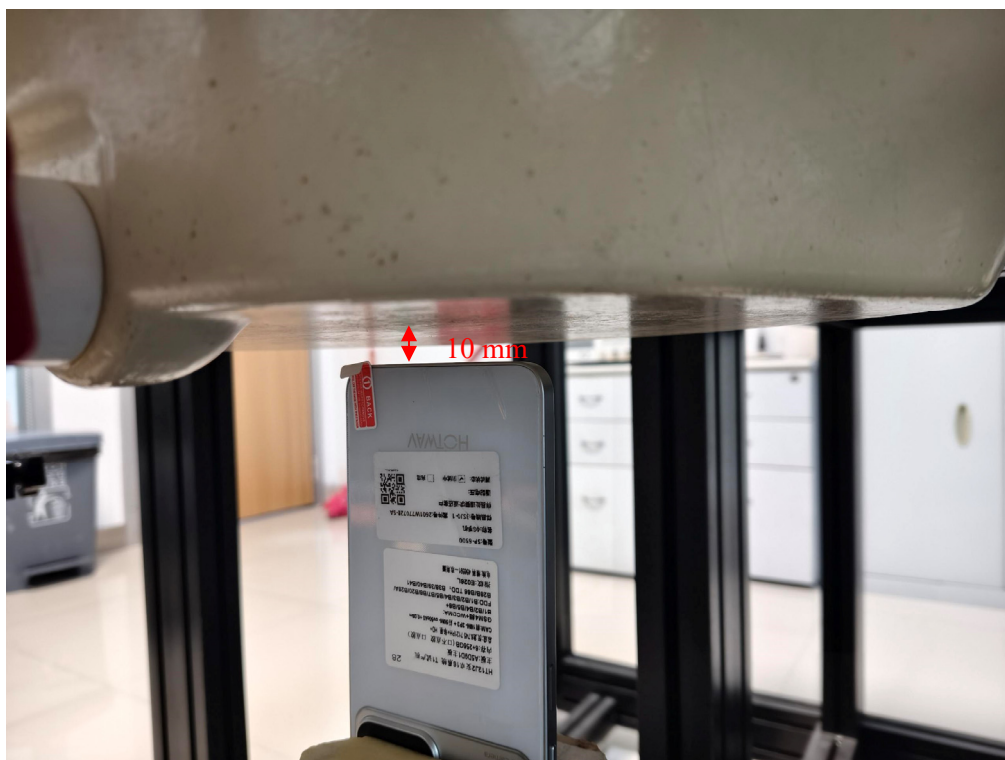
Body Bottom Setup Photo (10 mm)
