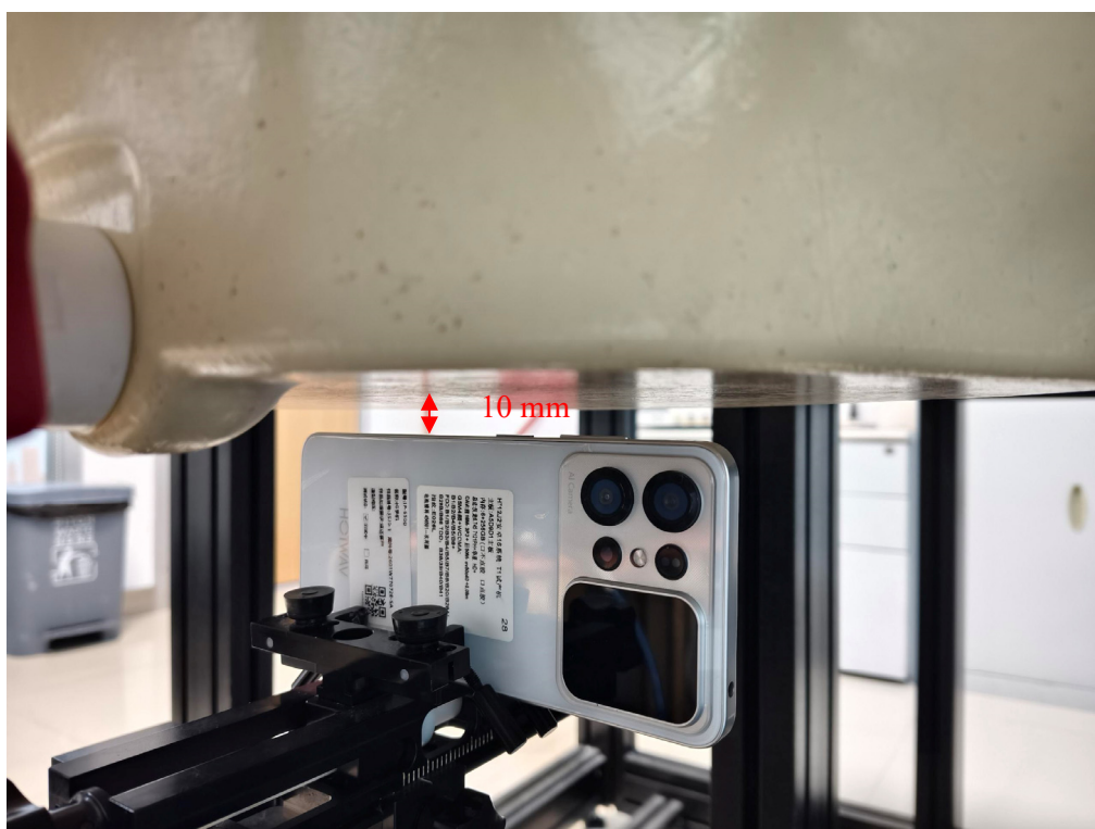
Body Right Setup Photo (10 mm)
