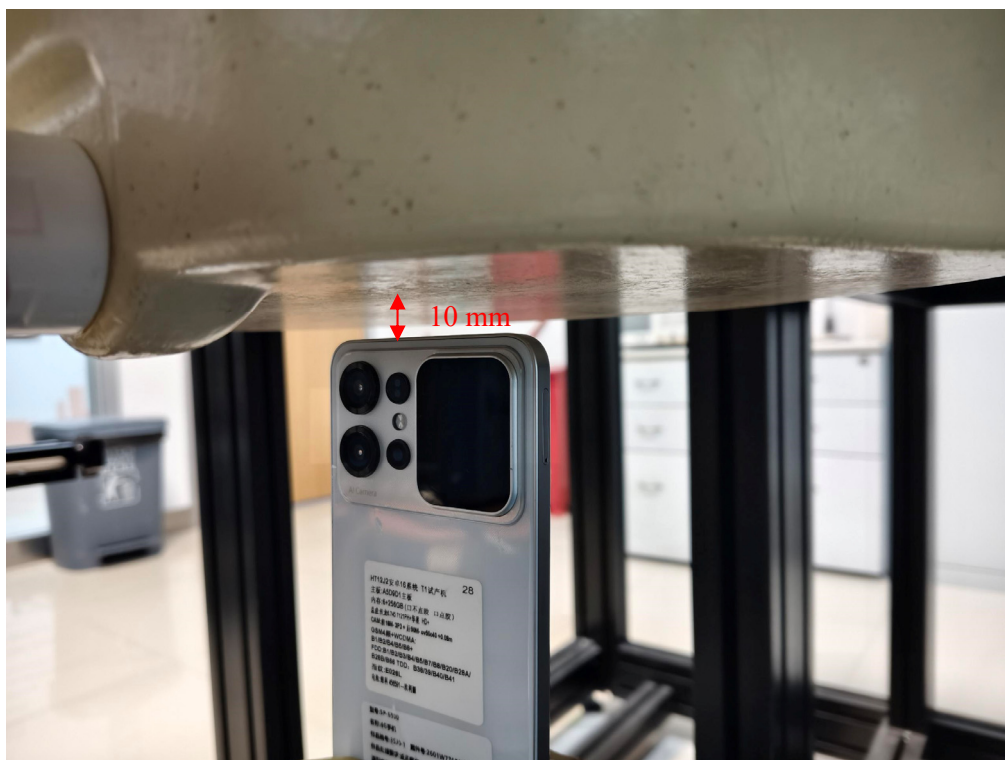
Body Top Setup Photo (10 mm)
