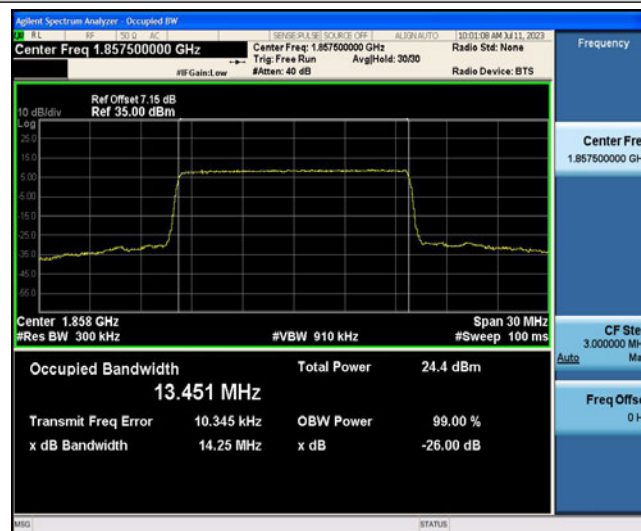
Band2-15MHz-16QAM-18900-75RB#0
