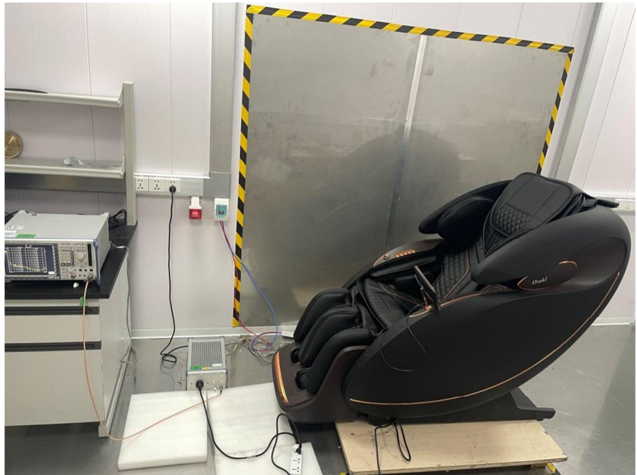
Conducted Emission Test Setup
