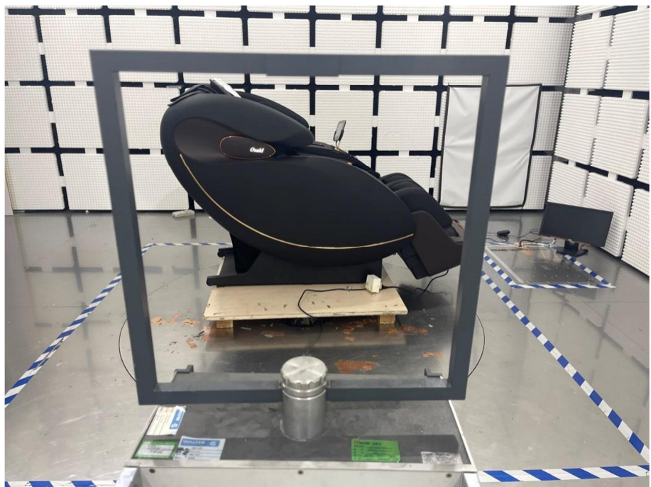
Radiation Emission Test Setup (Below 30MHz)
