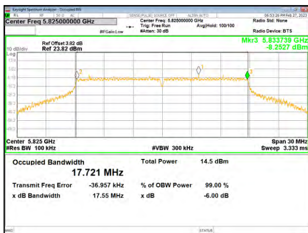
(802.11ac20) plot on channel 165
