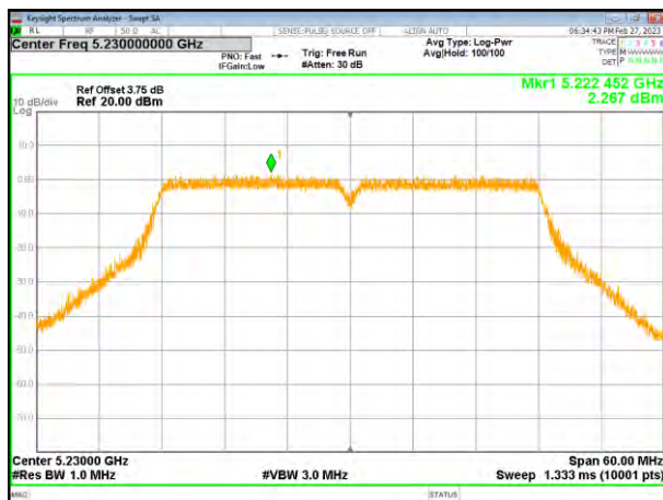
(802.11ac40) PSD plot on channel 46
