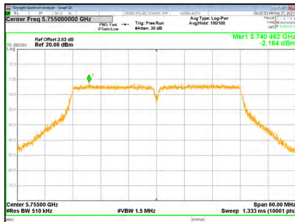
(802.11n40) PSD plot on channel 159
