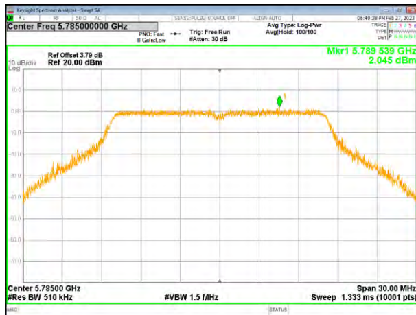
(802.11a) PSD plot on channel 157
