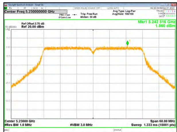
(802.11n40) PSD plot on channel 46
