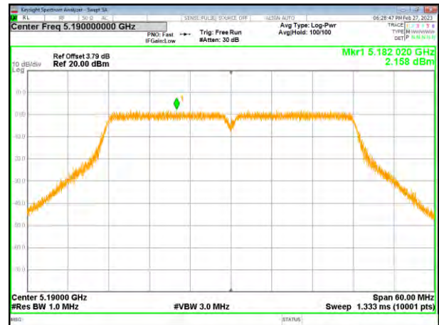
(802.11n40) PSD plot on channel 46
