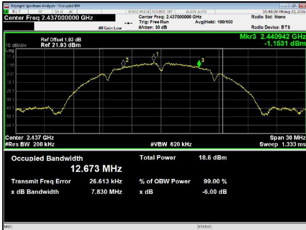
-6dB Bandwidth NVNT b 2437MHz Ant1
