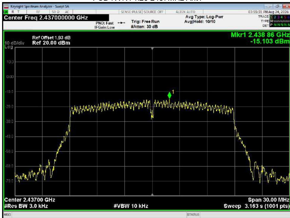
PSD NVNT n20 2437MHz Ant1
