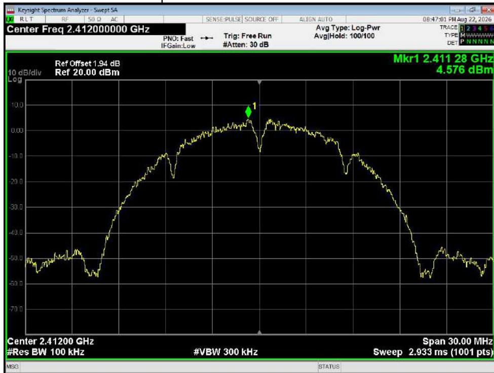
Tx. Spurious NVNT b 2412MHz Ant1 Emission
