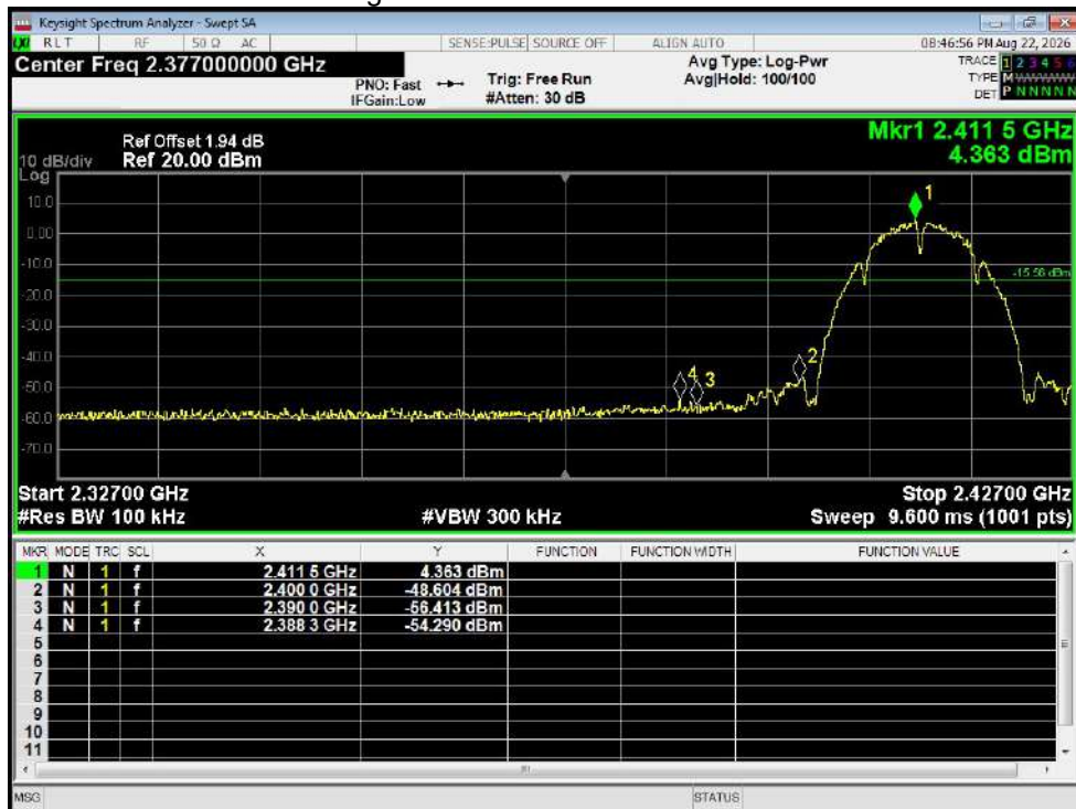
Band Edge NVNT b 2412MHz Ant1 Emission
