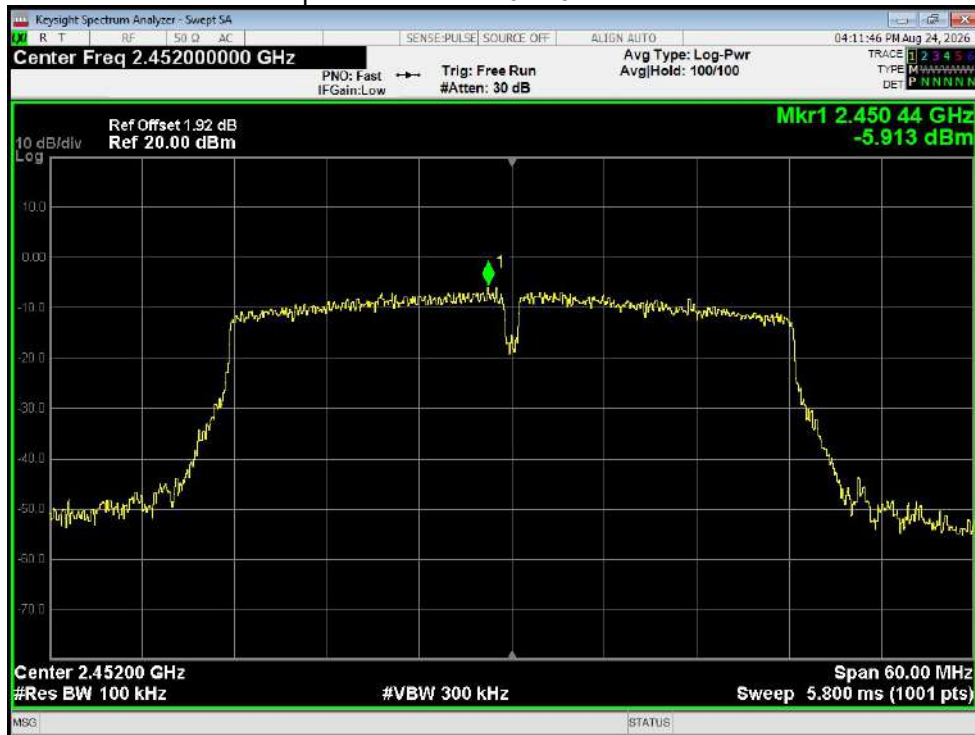
Tx. Spurious NVNT n40 2452MHz Ant1 Emission
