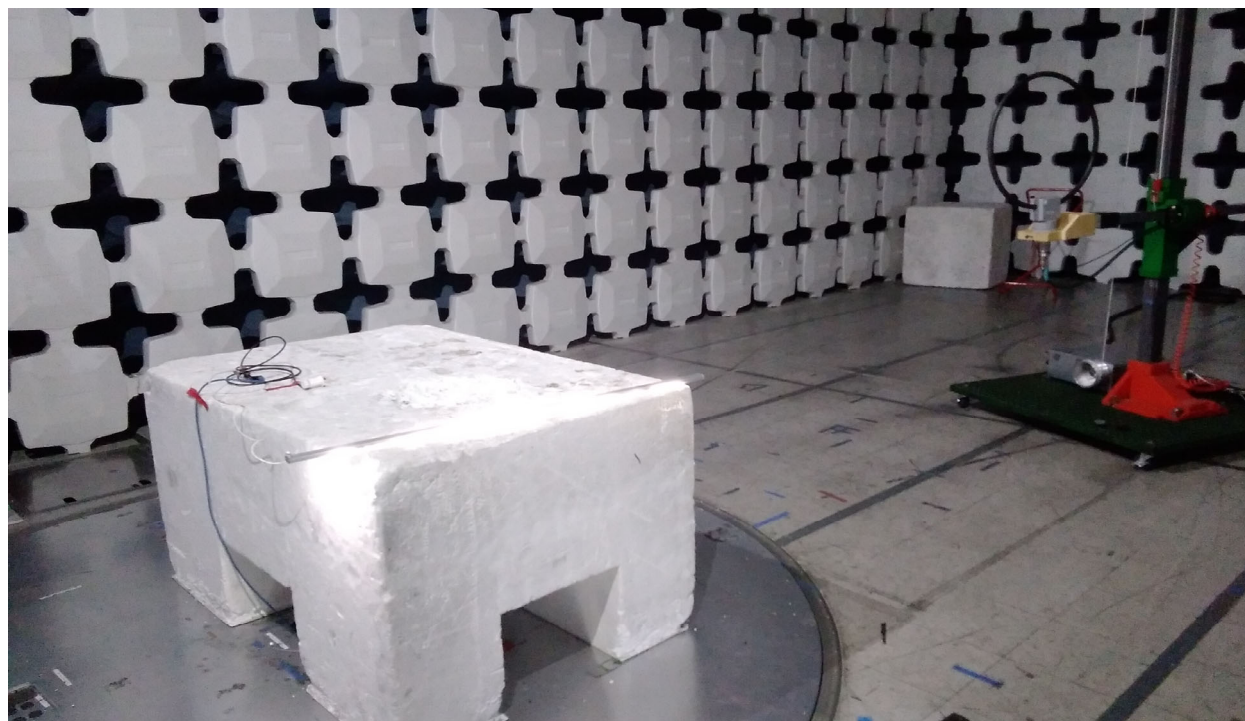
Test Configuration Photograph #2 (Radiated Emissions - Below 30 MHz)
