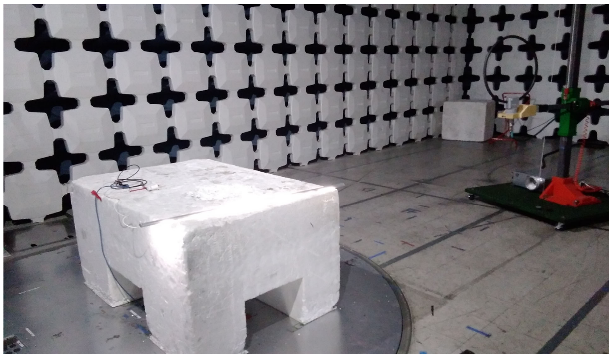
Test Configuration Photograph #1 (Radiated Emissions - Below 30 MHz)
