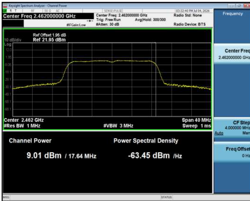
Average Power NVNT n20 2462MHz Ant1
