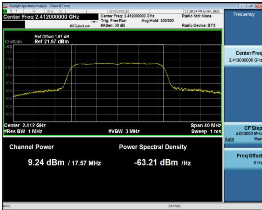
Average Power NVNT n20 2412MHz Ant1
