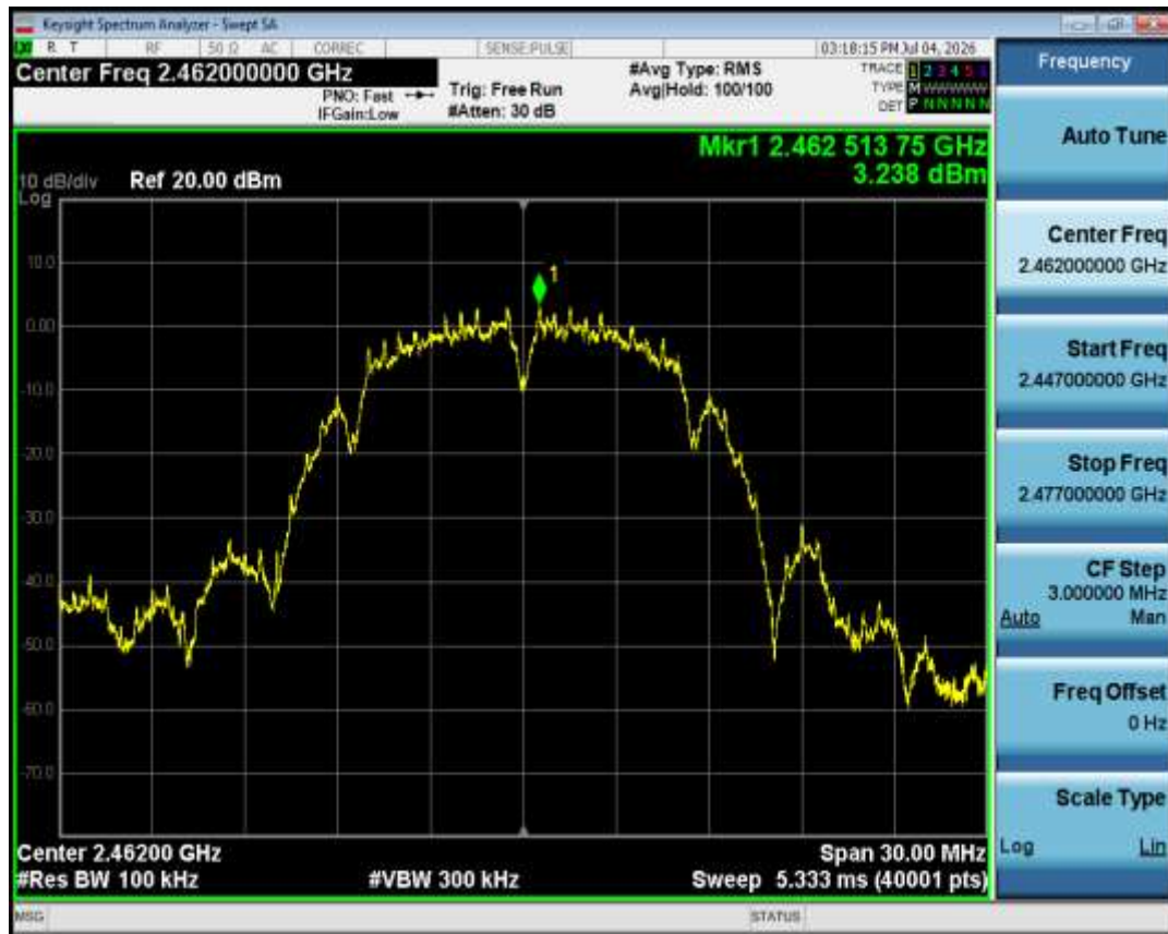
Tx. Spurious NVNT b 2462MHz Ant1 Ref
