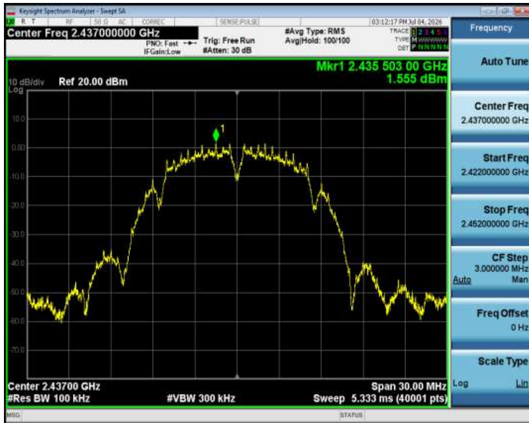
Tx. Spurious NVNT b 2437MHz Ant1 Ref
