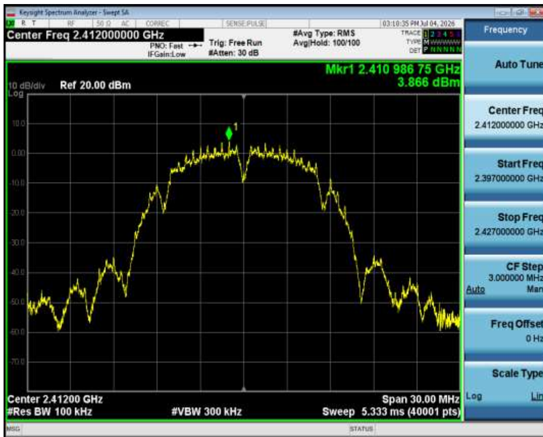
Tx. Spurious NVNT b 2412MHz Ant1 Ref
