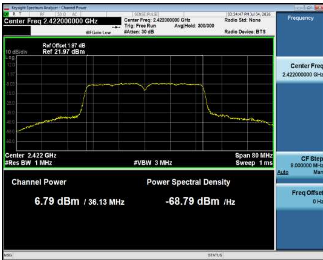
Average Power NVNT n40 2422MHz Ant1
