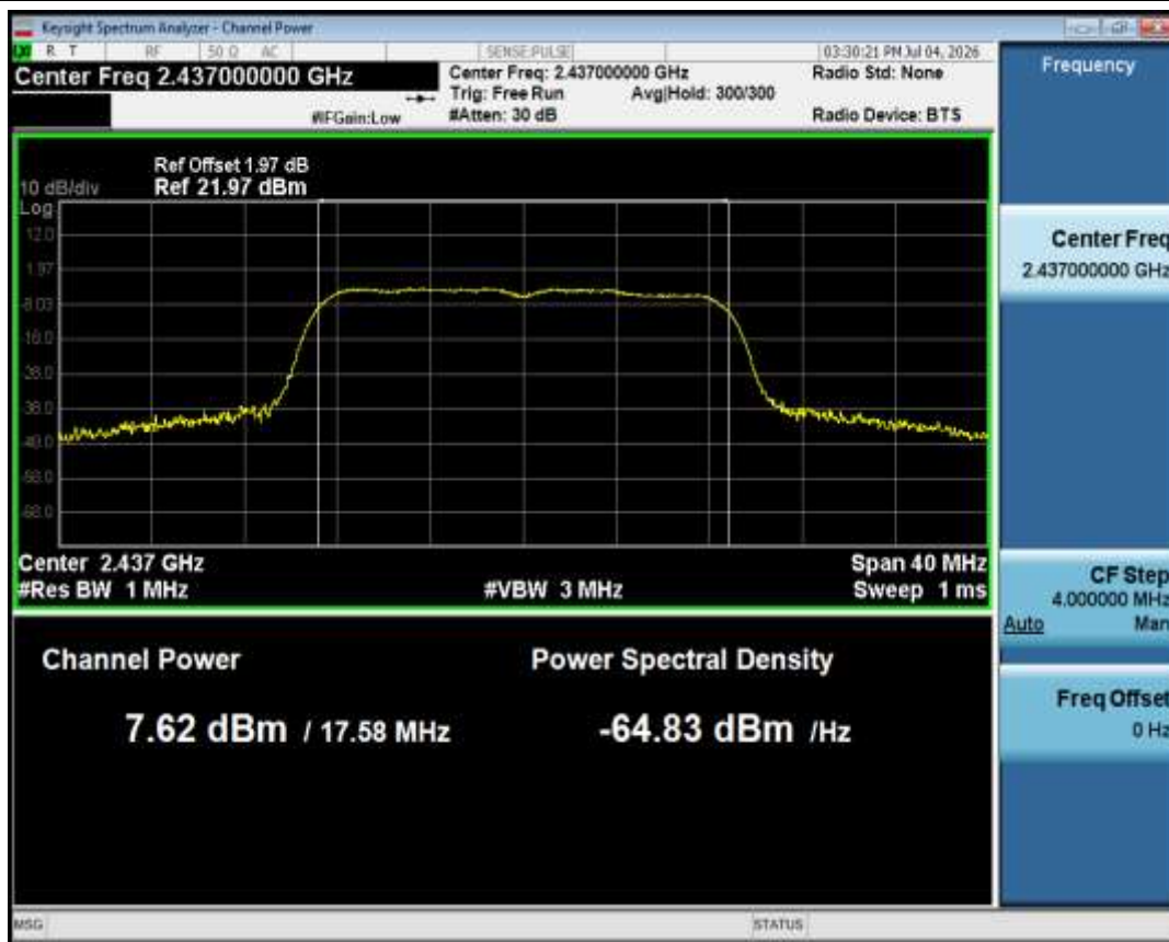
Average Power NVNT n20 2437MHz Ant1
