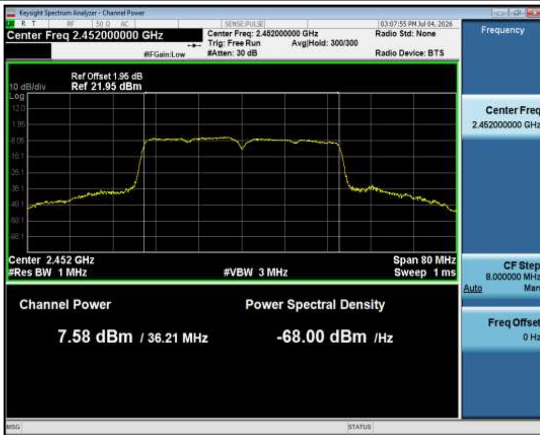
Average Power NVNT n40 2452MHz Ant1
