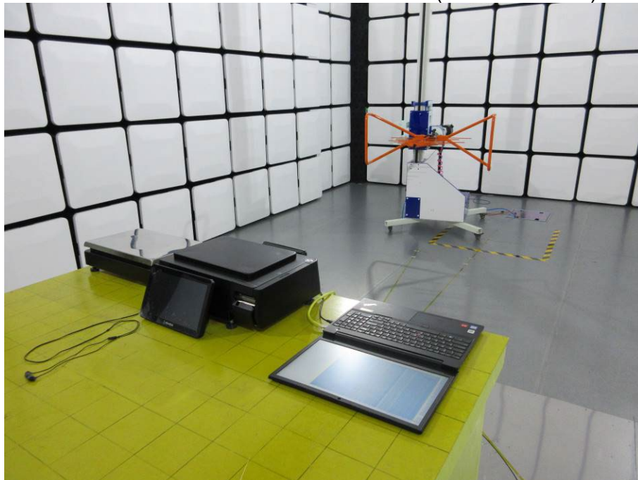
RADIATED RF MEASUREMENT SETUP (30MHz ~ 1 GHz)
