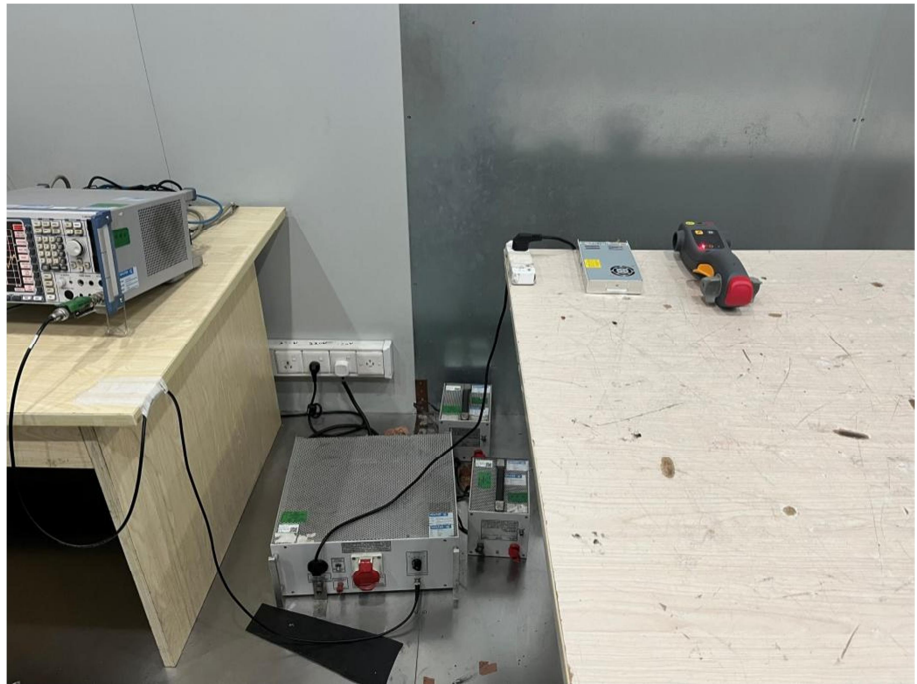
Conducted Emission Test Setup
