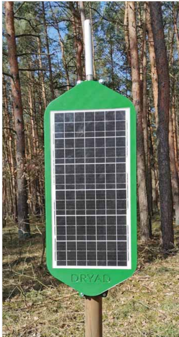
Mesh Gateway deployed on pole
