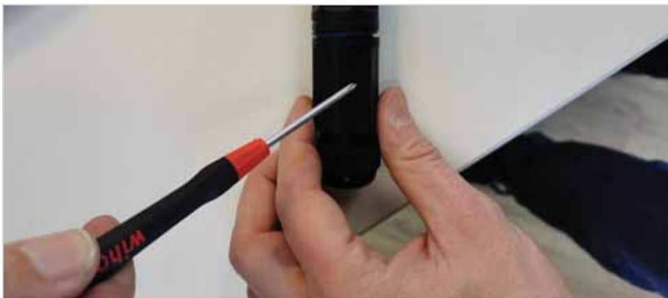
Border Gateway open Ethernet connector
