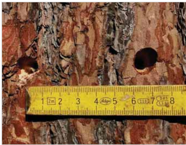
Drill two holes space 7 cm apart
