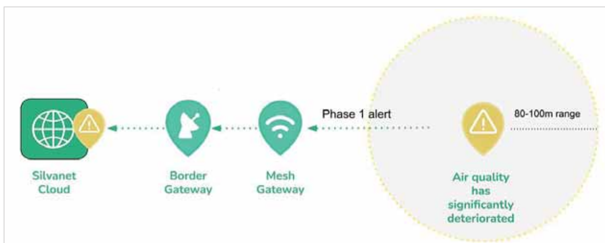
Step 3: Deterioration of air quality triggers Phase 1 alert
