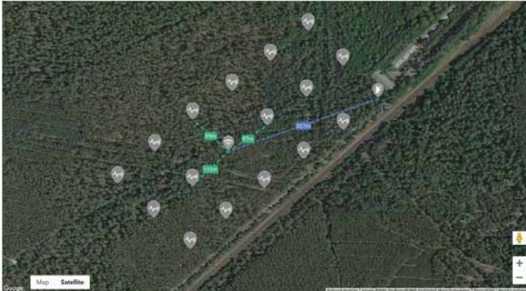
Placing Mesh Gateways
