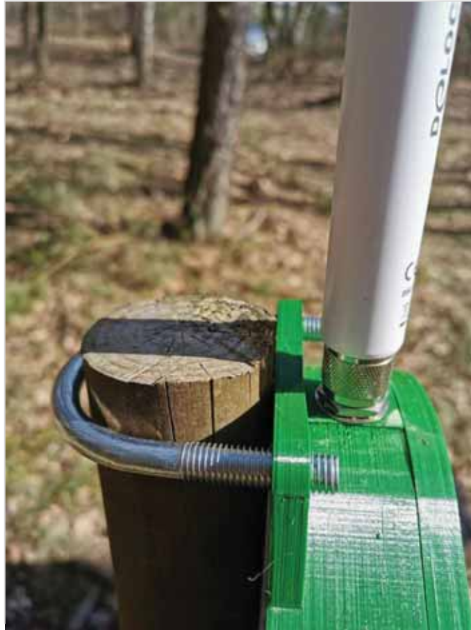
Border Gateway to a pole using a clamp
