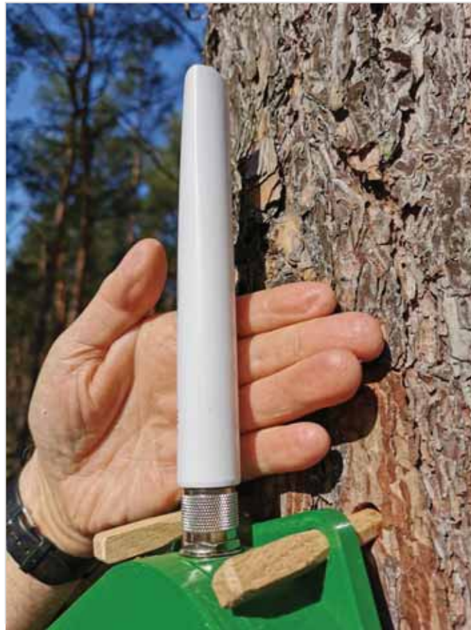
Finger width distance from tree
