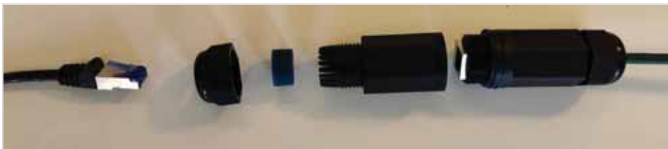
Border Gateway disassemble Ethernet connector
