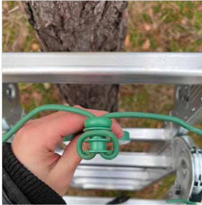
Insert crop wire through sensor and spacer
