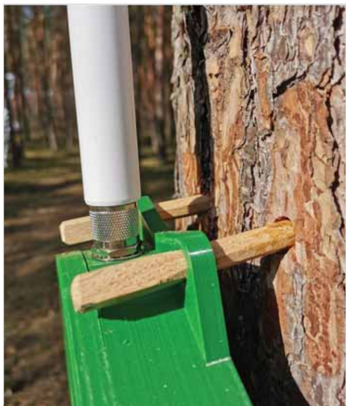
Mesh Gateway attached at the top
