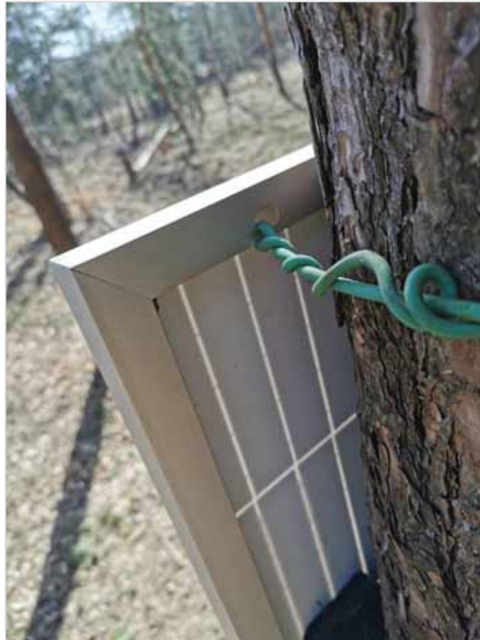
Solar panel attached using crop wire
