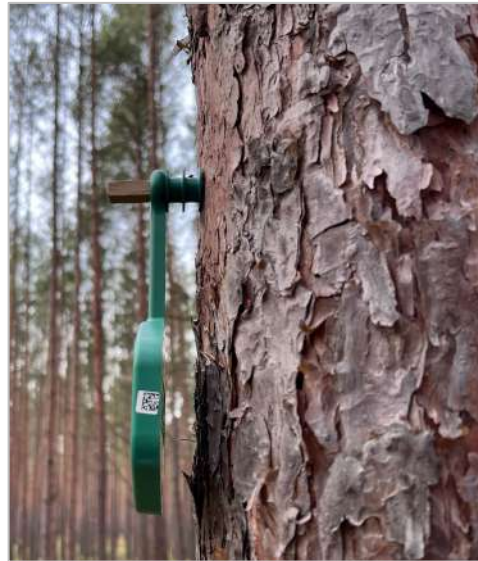
Attached sensor using tree nail
