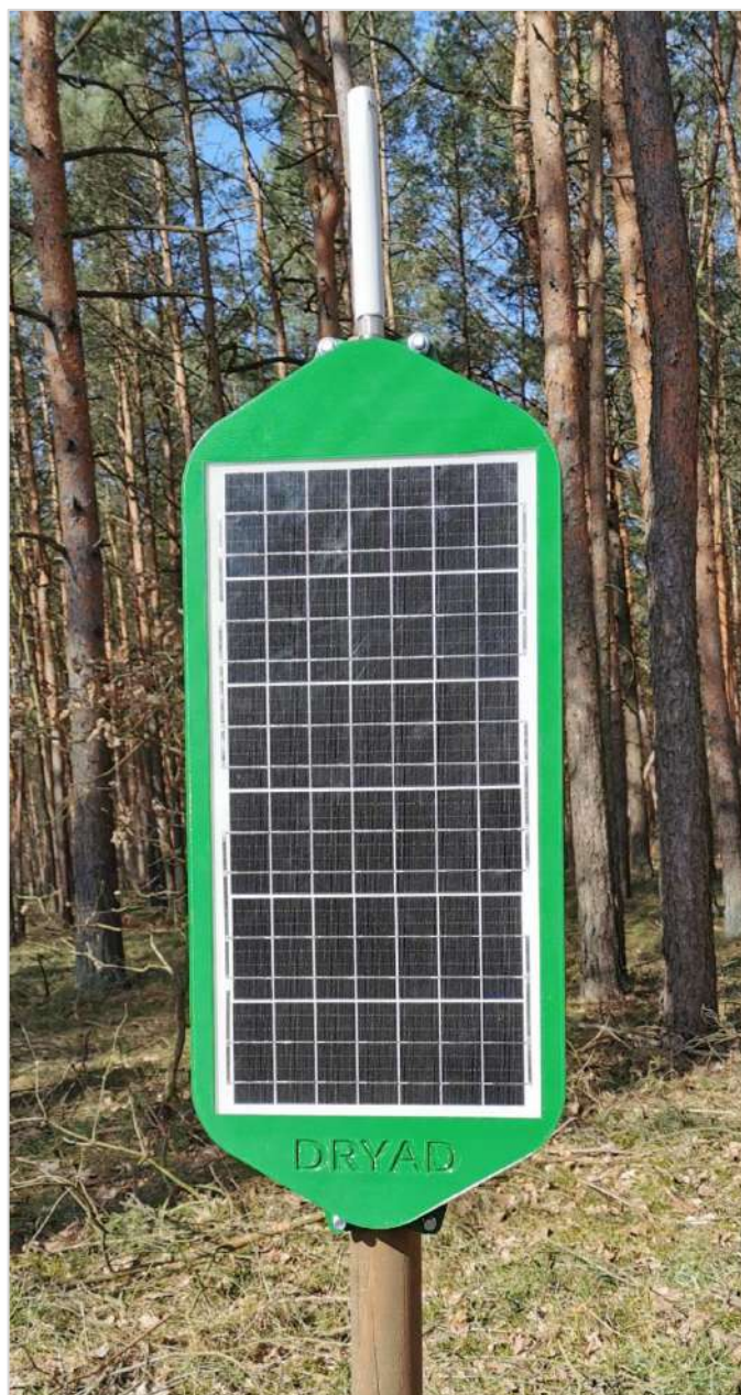
Mesh Gateway deployed on pole
