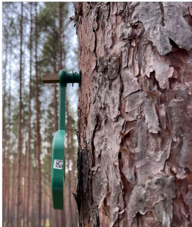
Sensor attached with treenail and spacer
