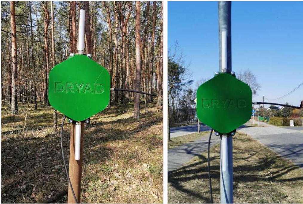
Border Gateway deployed on a pole
