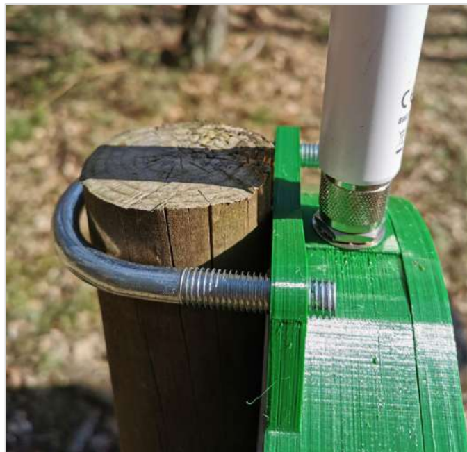
Arrange clamps around pole
