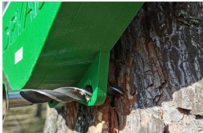
Drill the bottom two holes
