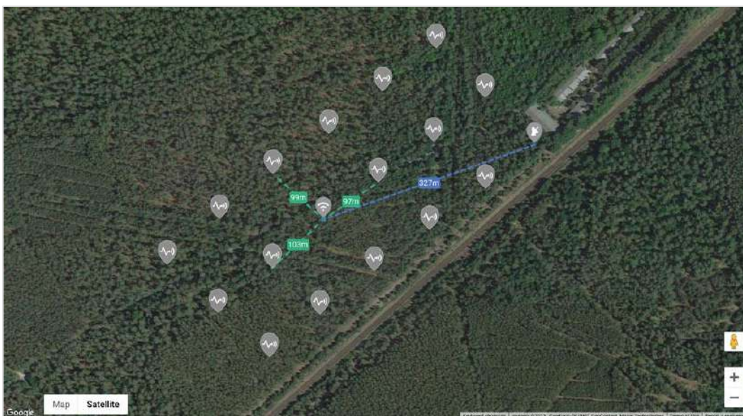
Placing Mesh Gateways
