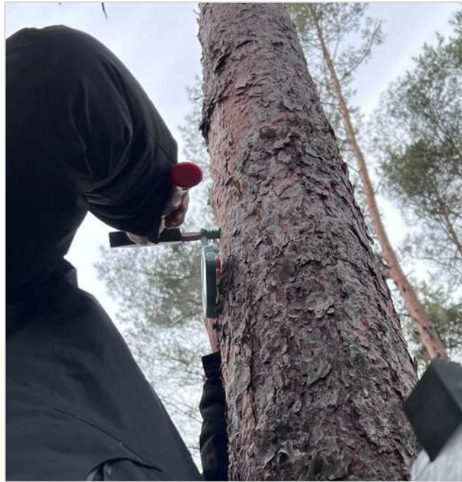
Hammer in treenail through sensor and spacer
