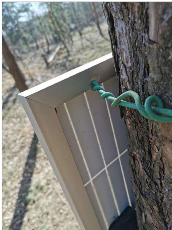
Solar panel attached using crop wire
