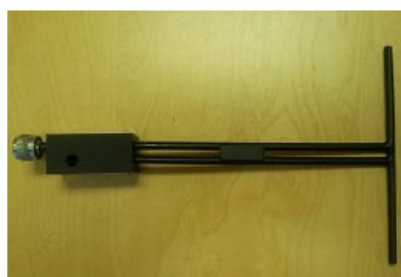
Figure 1 – MVG COMOSAR Validation Dipole
