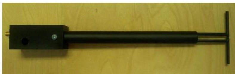
Figure 1 – MVG COMOSAR Validation Dipole
