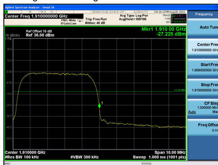
Higher Band Edge Plot on Channel 9538
