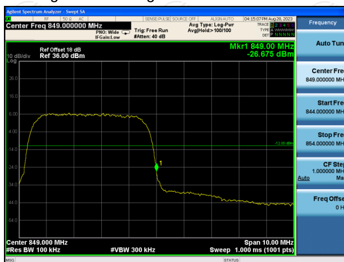
Higher Band Edge Plot on Channel 4233
