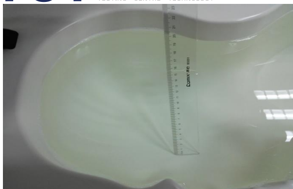
The Head Liquid of 1900MHz (15.5cm)
