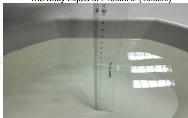
The Body Liquid of 5000-6000MHz (16.5cm)
