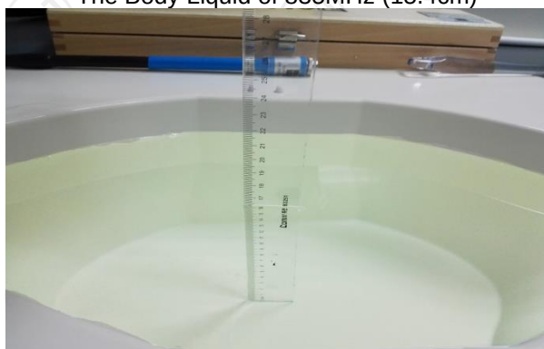
The Body Liquid of 1900MHz (16.4 cm)
