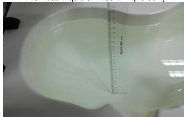
The Head Liquid of 1800MHz (15.2cm)
