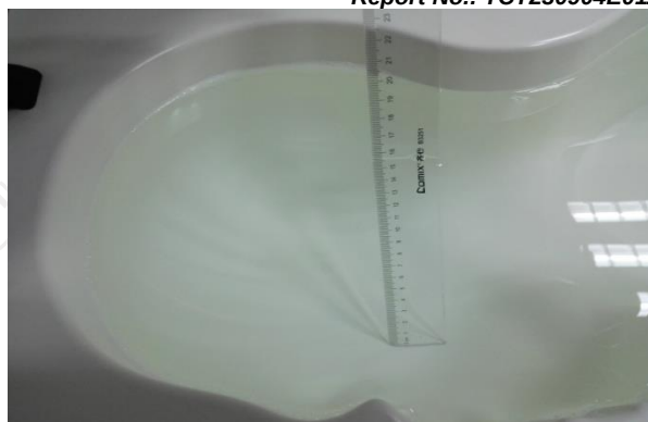
The Head Liquid of 2450MHz (15.6cm)
