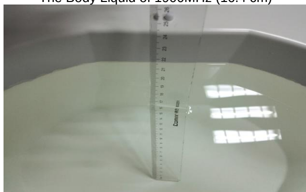
The Body Liquid of 2600MHz (16.5cm)
