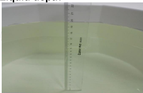
The Body Liquid of 835MHz (15.4cm)
