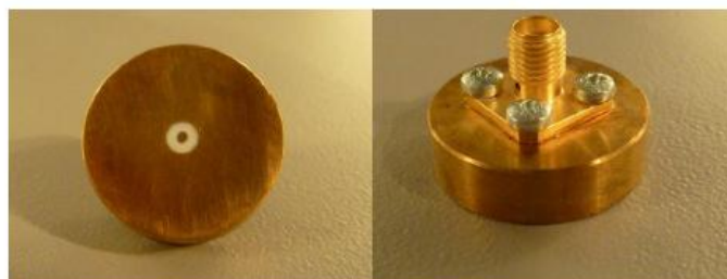
Figure 1 – MVG LIMESAR Dielectric Probe
