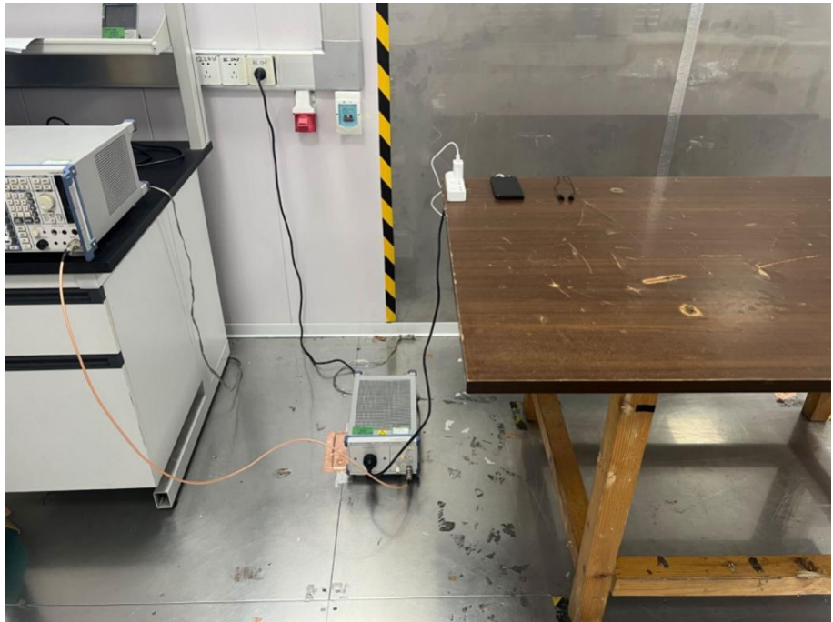
Conducted Emission Test Setup
