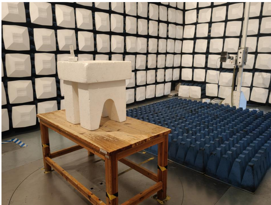
Test Setup For Radiated Emission (Above 1GHz)
