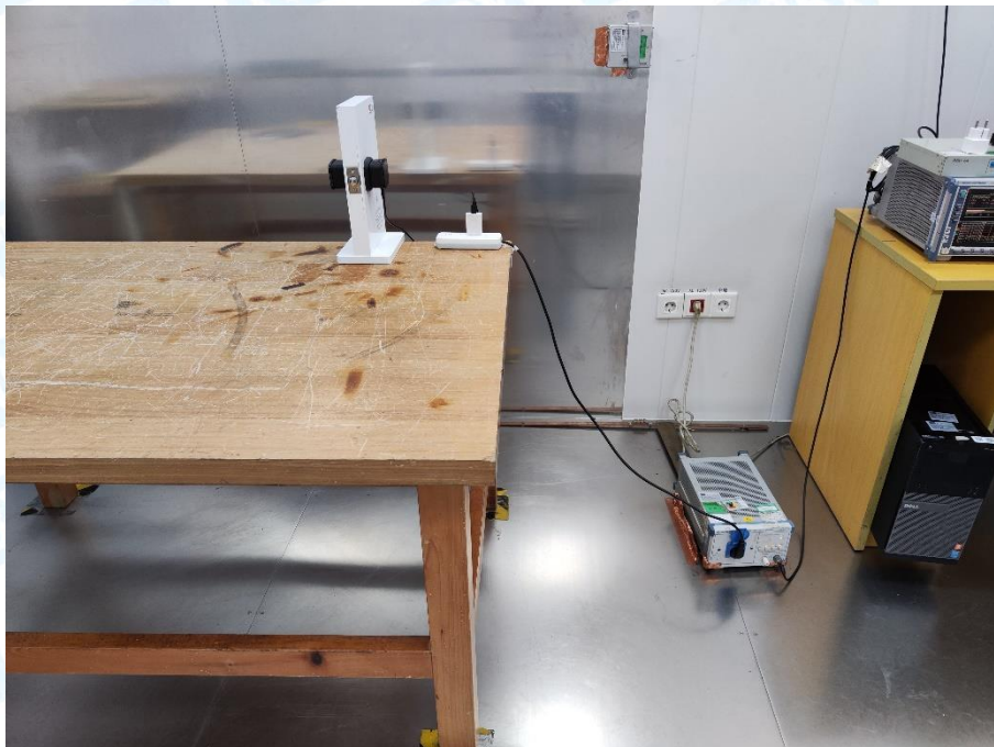
Photo of Setup for Conducted Emission
