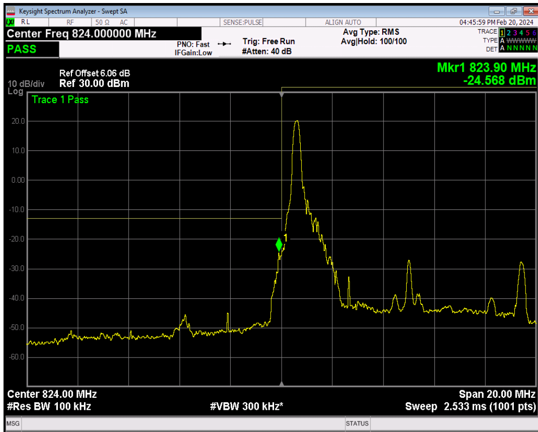
Band5 16QAM BW=10MHz Channel=20450 RB Size=1 Position=#Max
