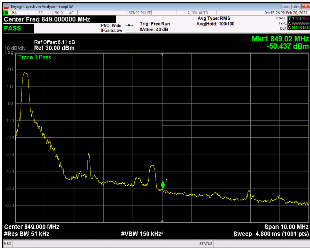
Band5 QPSK BW=5MHz Channel=20625 RB Size=1 Position=#Max
