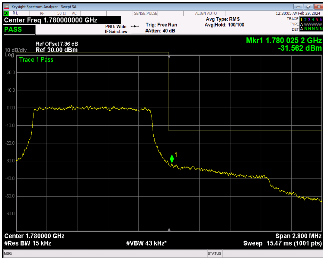
Band66 16QAM BW=1.4MHz Channel=132665 RB Size=1 Position=#0
