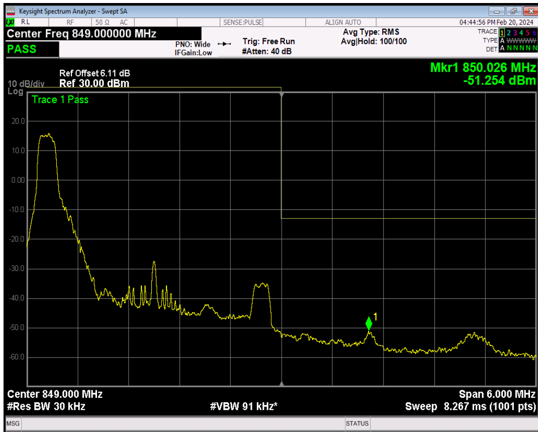
Band5 16QAM BW=3MHz Channel=20635 RB Size=1 Position=#Max
