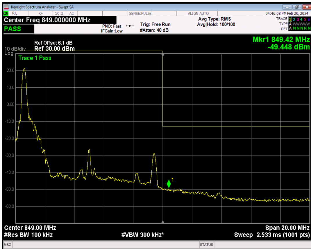
Band5 QPSK BW=10MHz Channel=20600 RB Size=1 Position=#Max
