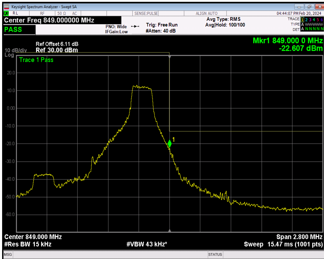
Band5 16QAM BW=1.4MHz Channel=20643 RB Size=6 Position=#0
