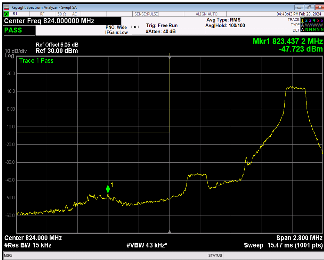
Band5 16QAM BW=1.4MHz Channel=20407 RB Size=6 Position=#0
