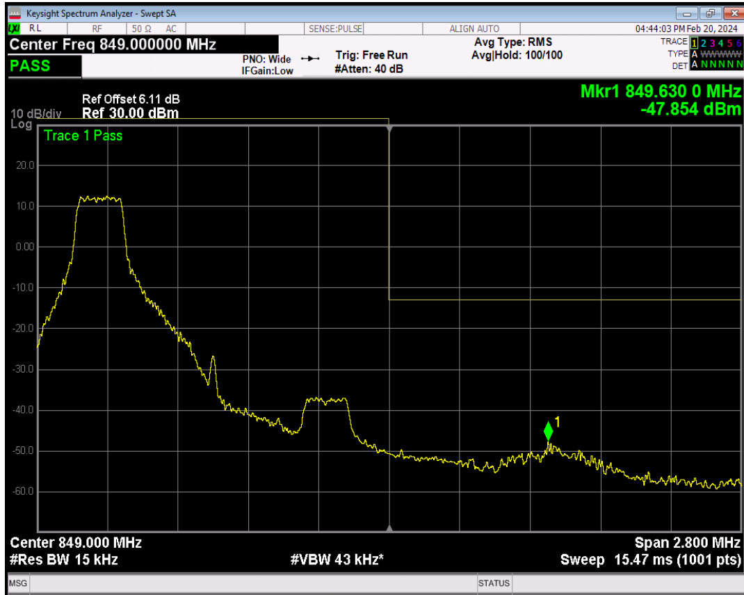
Band5 16QAM BW=1.4MHz Channel=20643 RB Size=1 Position=#Max
