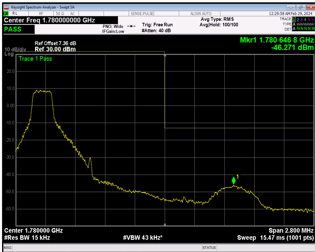
Band66 QPSK BW=1.4MHz Channel=132665 RB Size=1 Position=#Max
