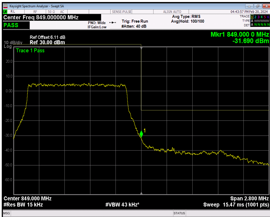
Band5 16QAM BW=1.4MHz Channel=20643 RB Size=1 Position=#0
