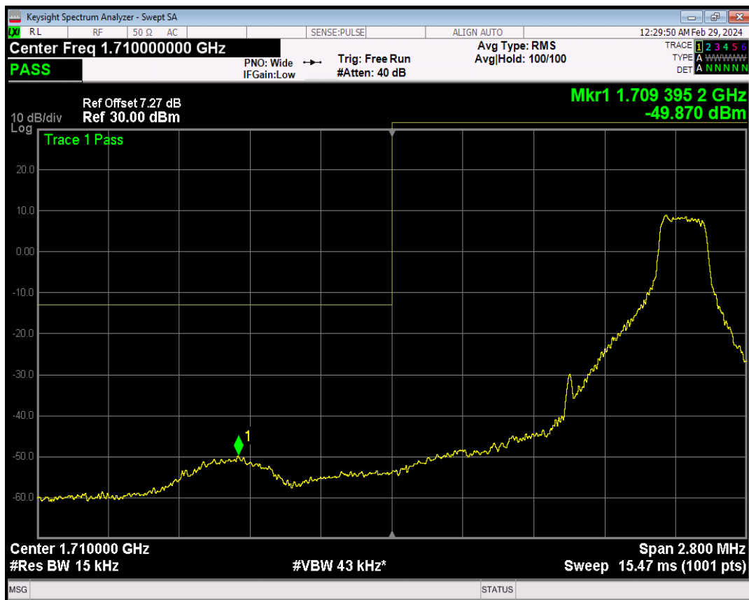
Band66 16QAM BW=1.4MHz Channel=131979 RB Size=6 Position=#0
