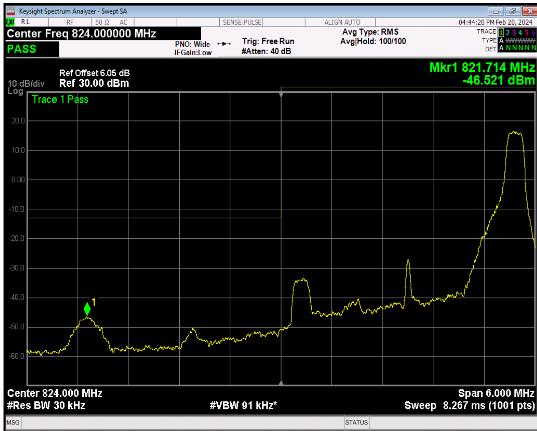
Band5 QPSK BW=3MHz Channel=20415 RB Size=15 Position=#0
