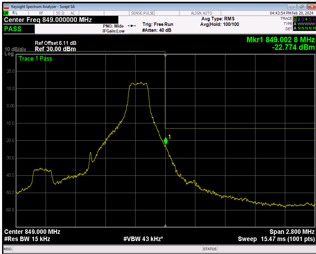
Band5 QPSK BW=1.4MHz Channel=20643 RB Size=6 Position=#0
