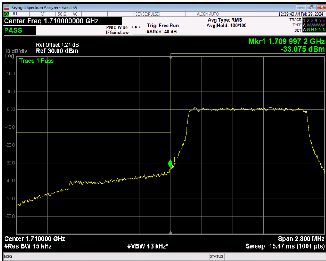
Band66 16QAM BW=1.4MHz Channel=131979 RB Size=1 Position=#0
