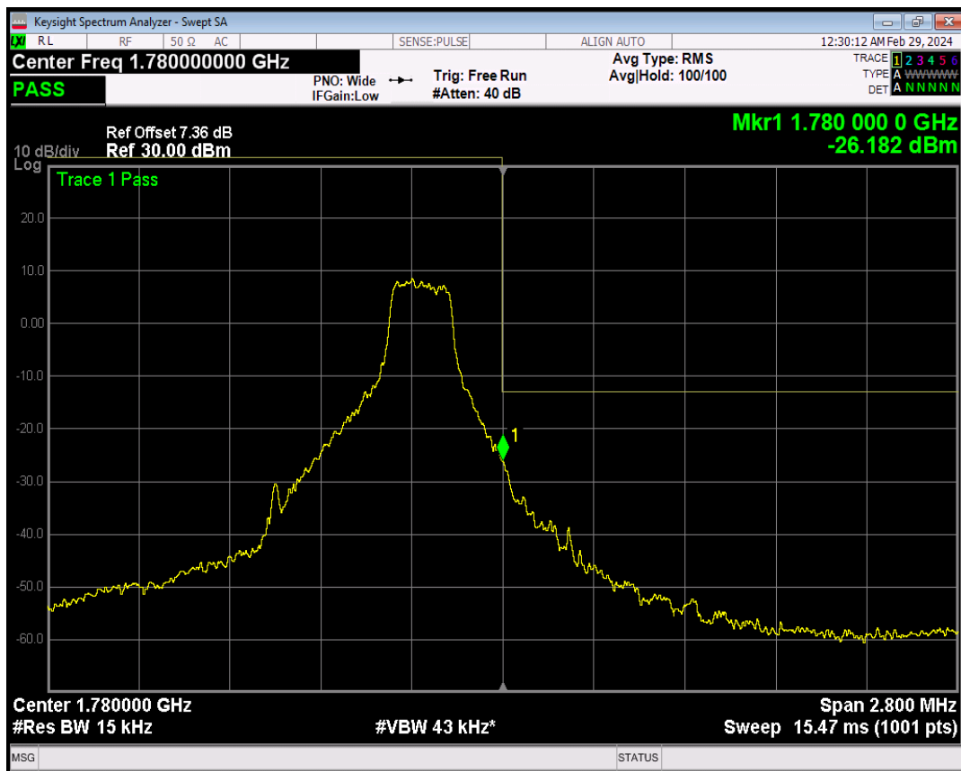
Band66 16QAM BW=1.4MHz Channel=132665 RB Size=6 Position=#0
