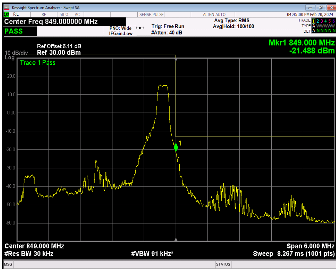
Band5 QPSK BW=5MHz Channel=20425 RB Size=1 Position=#0
