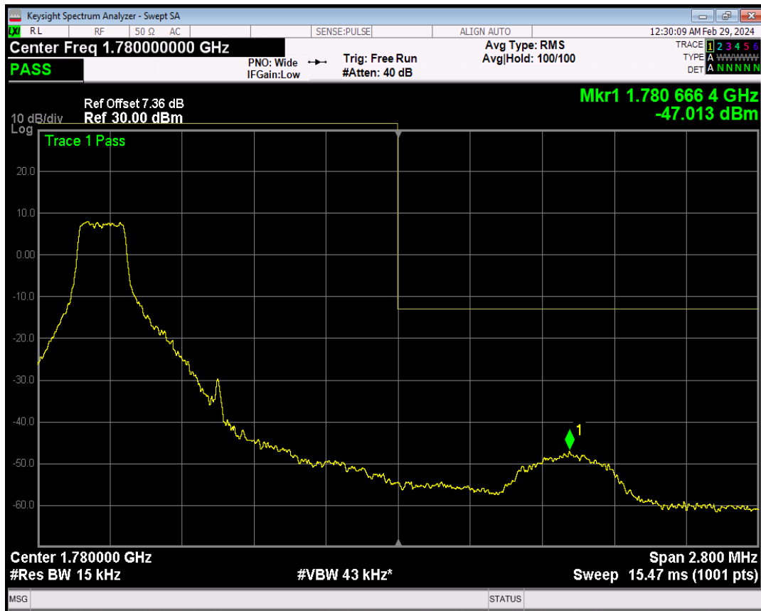
Band66 16QAM BW=1.4MHz Channel=132665 RB Size=1 Position=#Max
