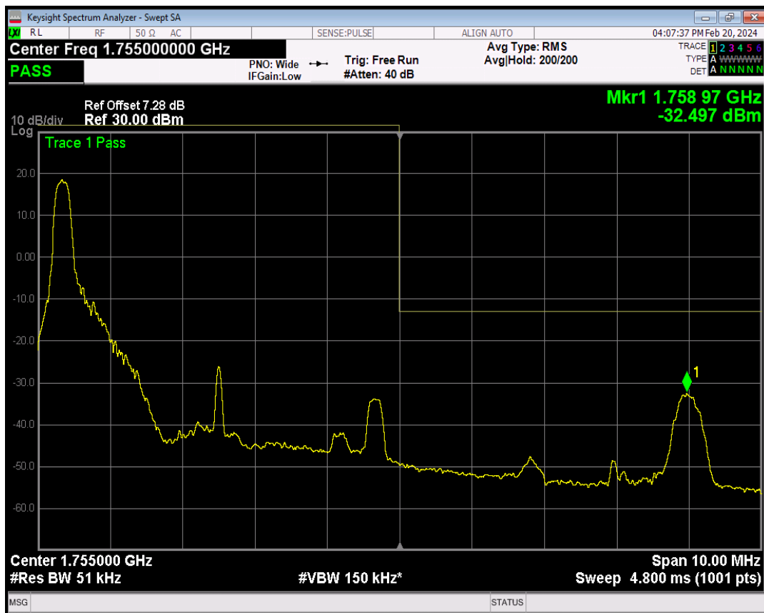
Band4 QPSK BW=5MHz Channel=20375 RB Size=1 Position=#Max
