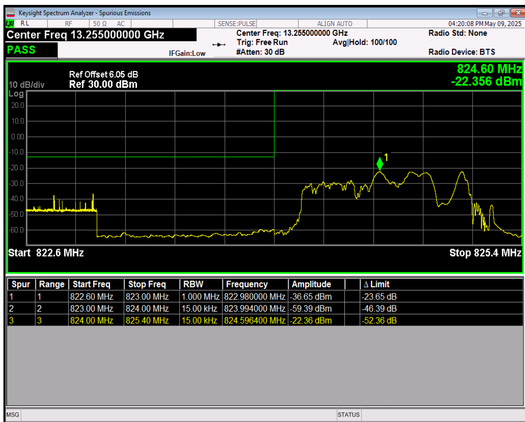
Band5 QPSK BW=1.4MHz Channel=20407 RB Size=6 Position=#0
