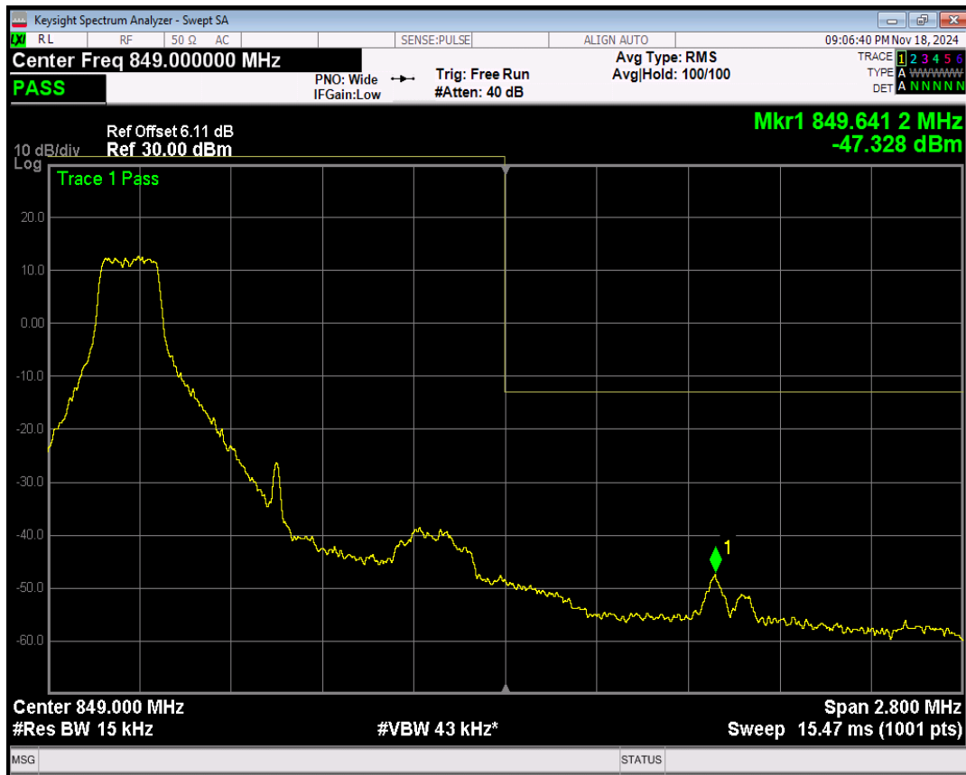
Band5 16QAM BW=1.4MHz Channel=20643 RB Size=1 Position=#Max
