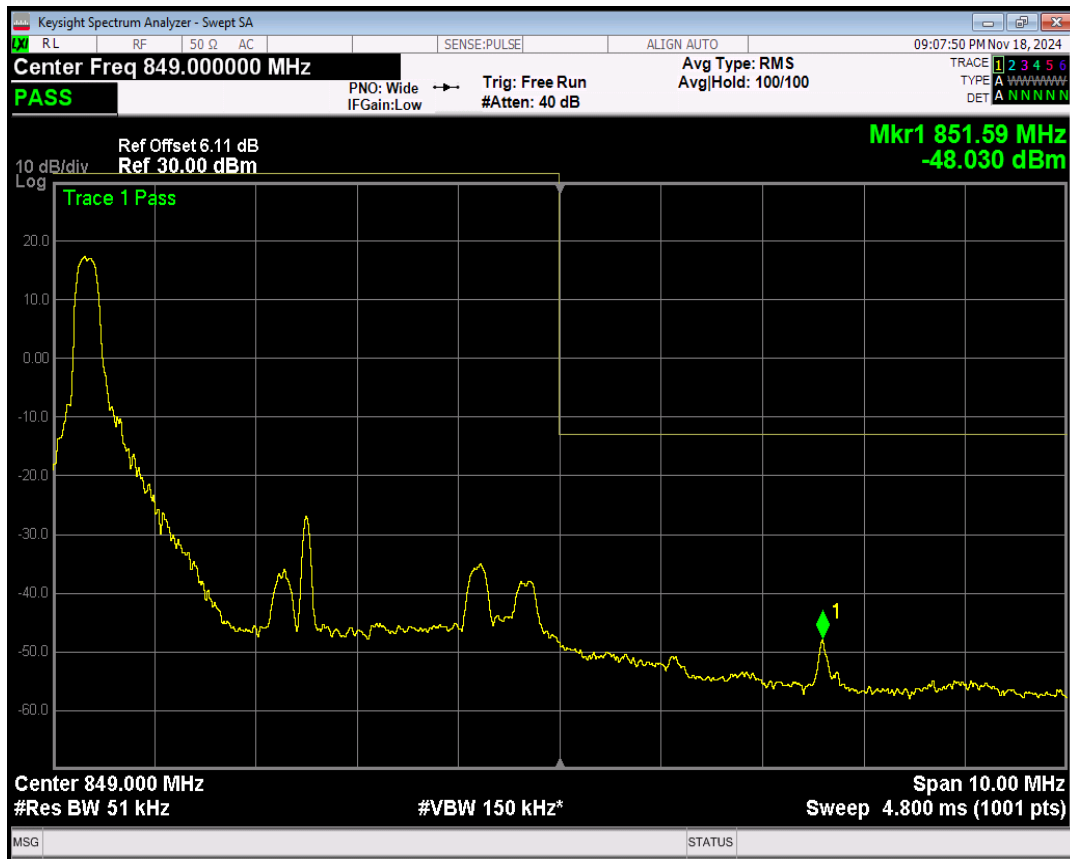
Band5 16QAM BW=5MHz Channel=20625 RB Size=1 Position=#Max
