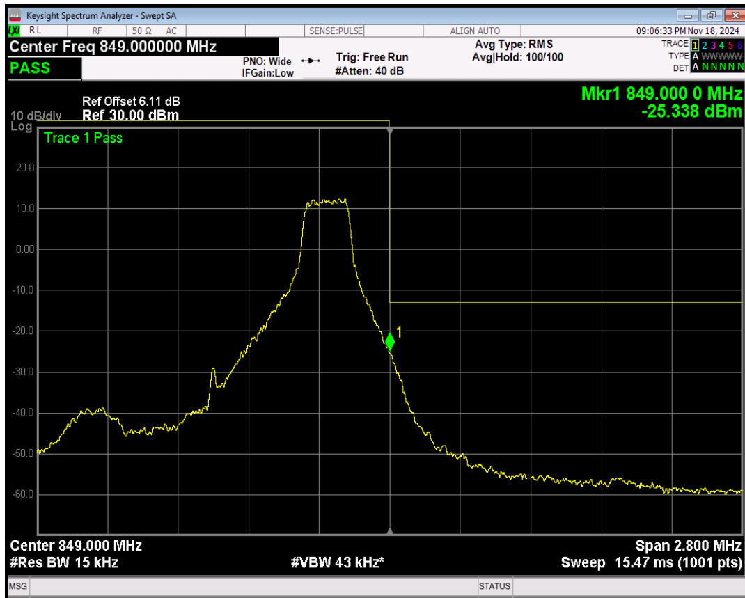
Band5 QPSK BW=1.4MHz Channel=20643 RB Size=6 Position=#0
