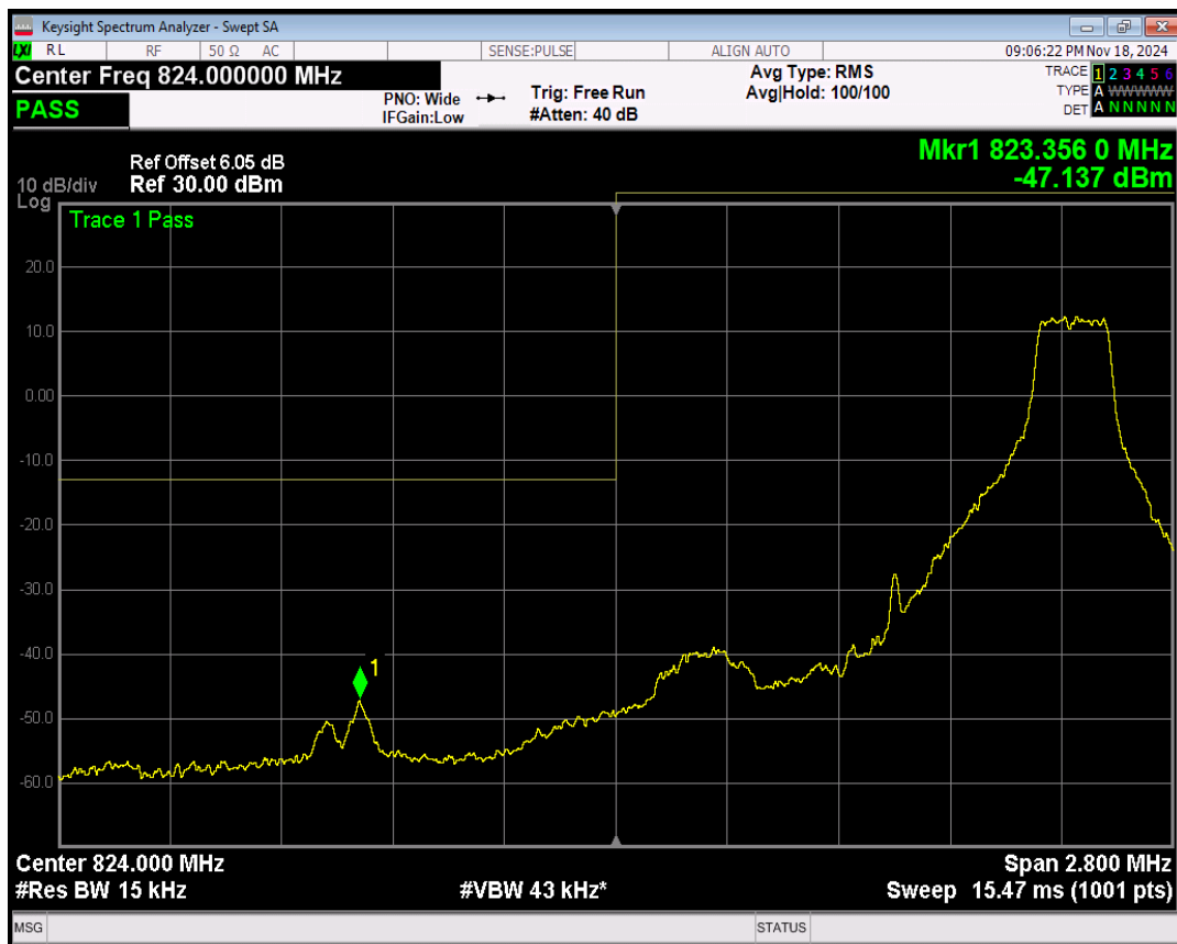
Band5 QPSK BW=1.4MHz Channel=20643 RB Size=1 Position=#0
