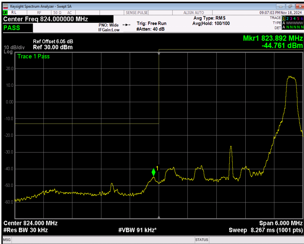
Band5 16QAM BW=3MHz Channel=20415 RB Size=15 Position=#0
