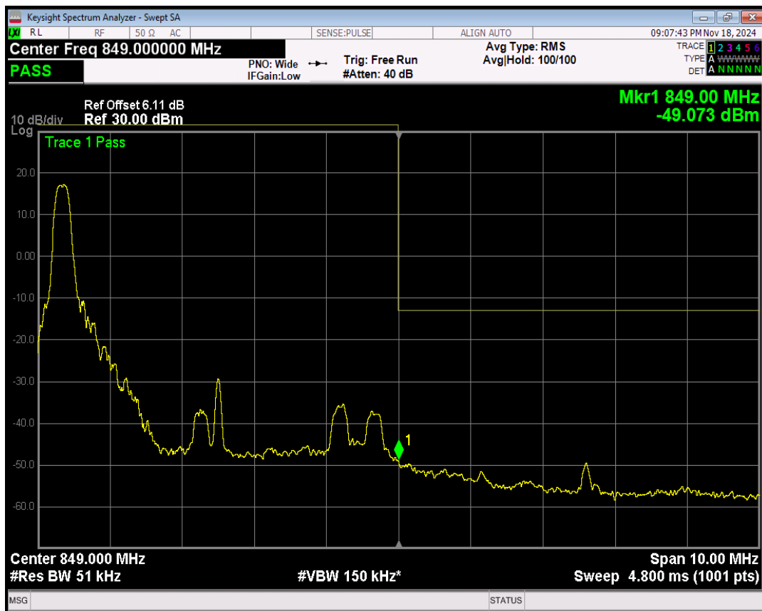
Band5 QPSK BW=5MHz Channel=20625 RB Size=1 Position=#Max
