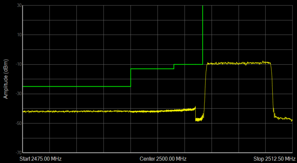
Band7 QPSK BW=10MHz Channel=20800 RB Size=50 Position=#0
