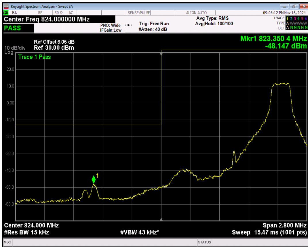
Band5 QPSK BW=1.4MHz Channel=20407 RB Size=6 Position=#0
