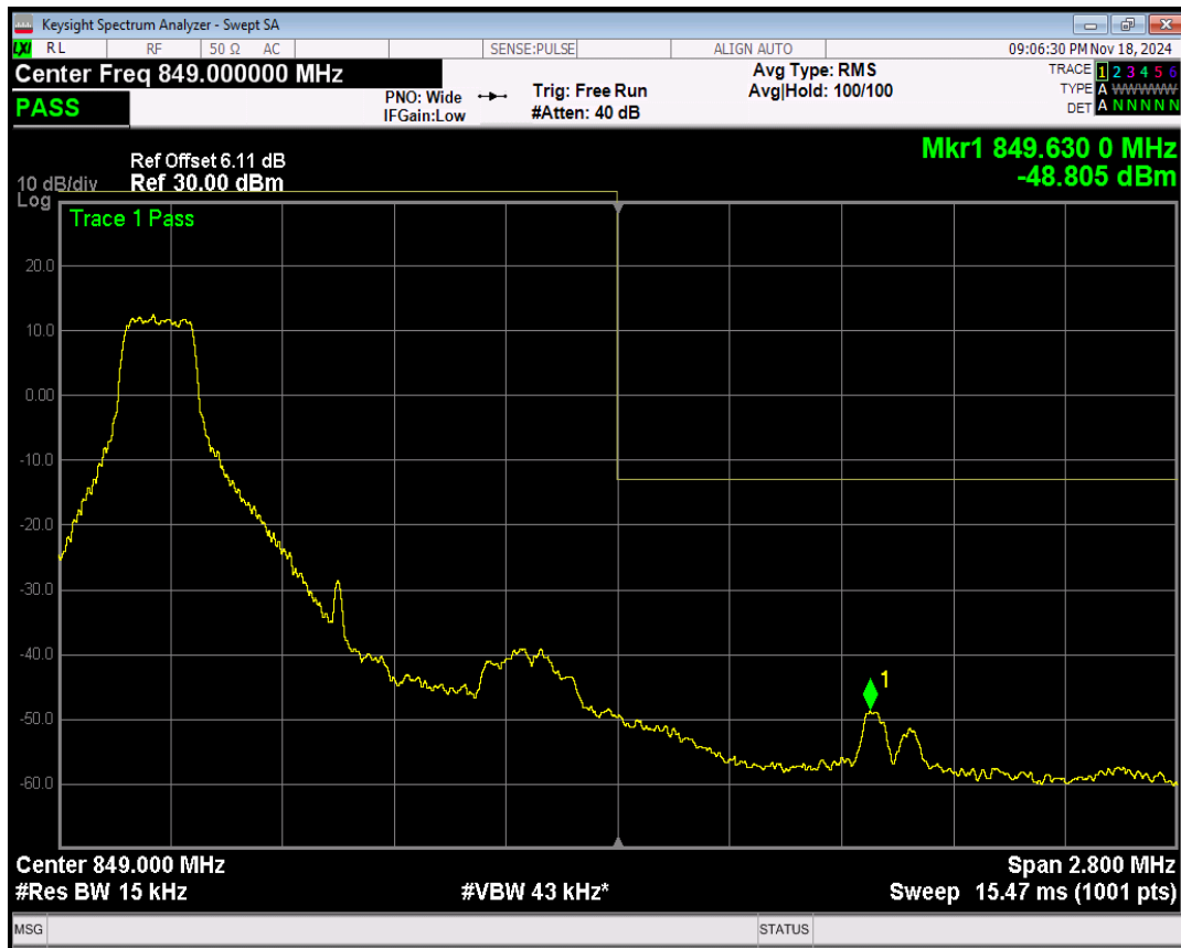
Band5 16QAM BW=1.4MHz Channel=20407 RB Size=6 Position=#0
