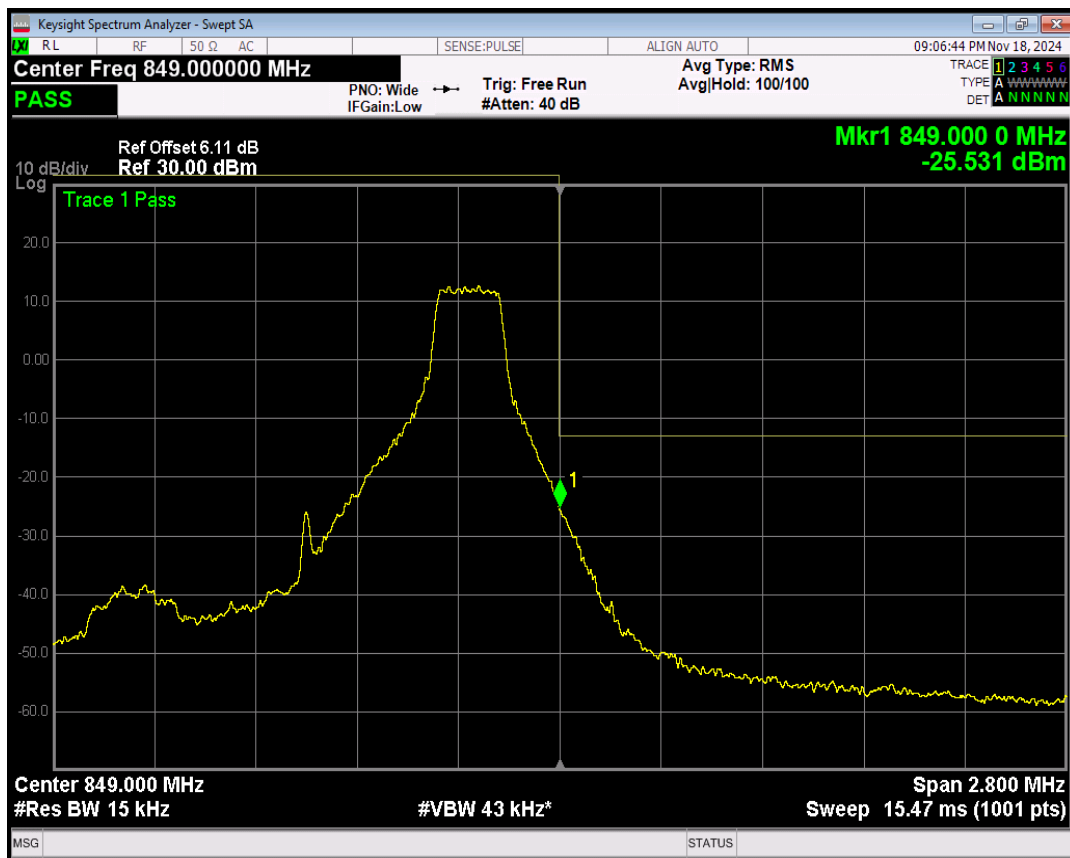
Band5 16QAM BW=1.4MHz Channel=20643 RB Size=6 Position=#0
