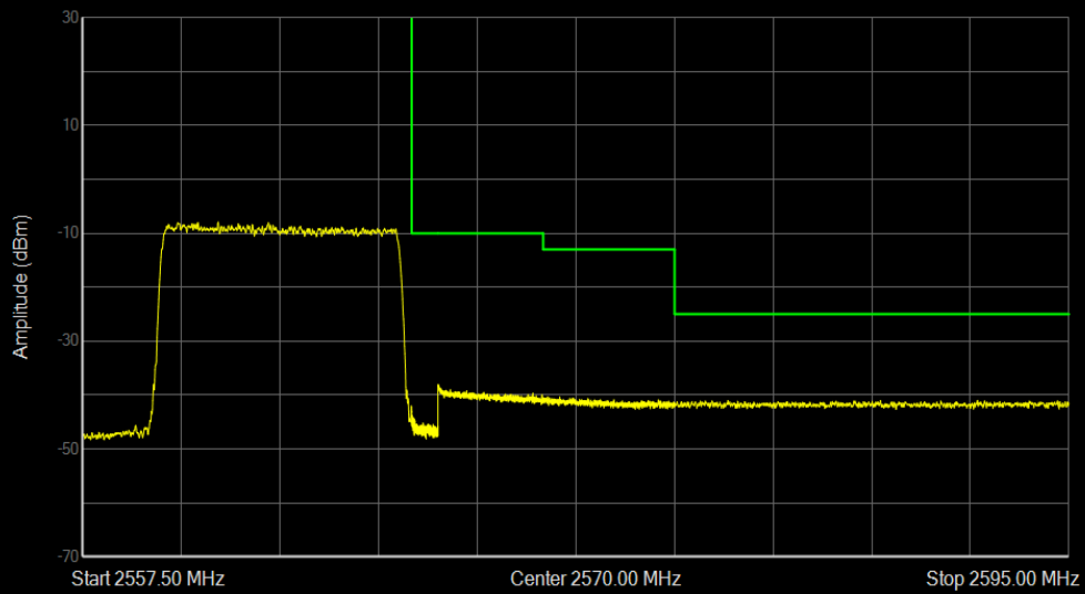
Band7 QPSK BW=10MHz Channel=21400 RB Size=50 Position=#0
