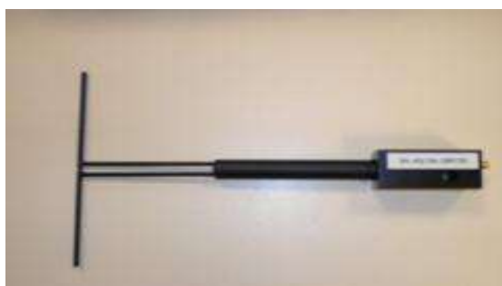
Figure 1 – MVG COMOSAR Validation Dipole
