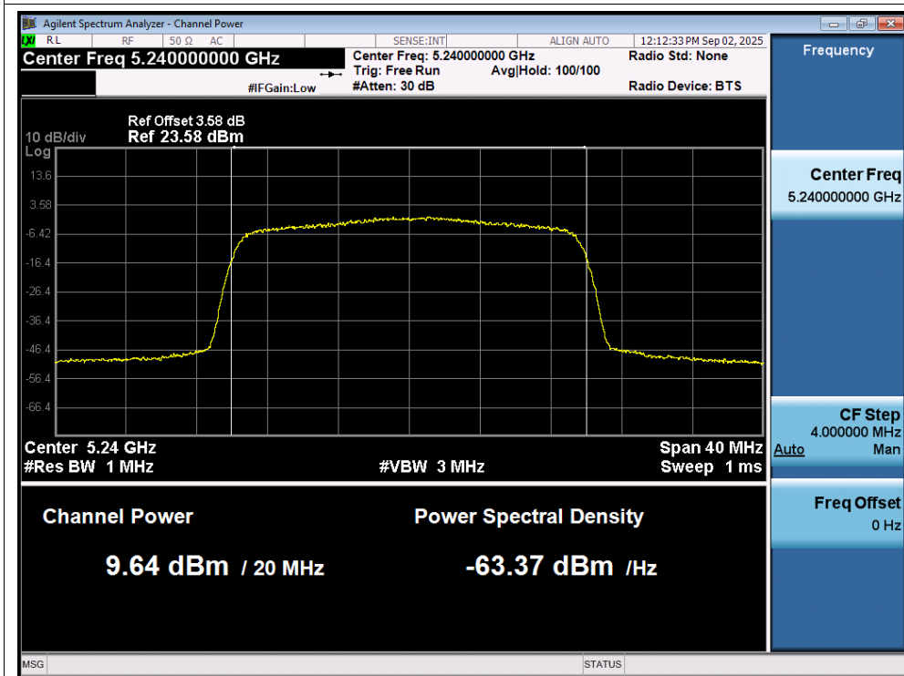
Power NVNT ax40 5190MHz AntA
