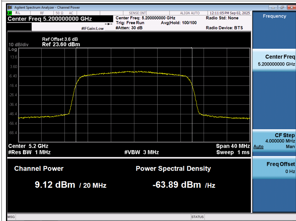
Power NVNT ax20 5200MHz AntA
