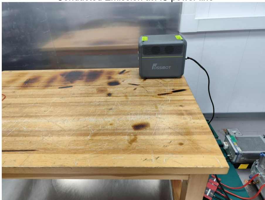
Conducted Emission at AC power line
