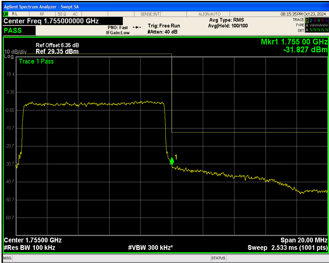
Band4 16QAM BW=10MHz Channel=20350 RB Size=50 Position=#0
