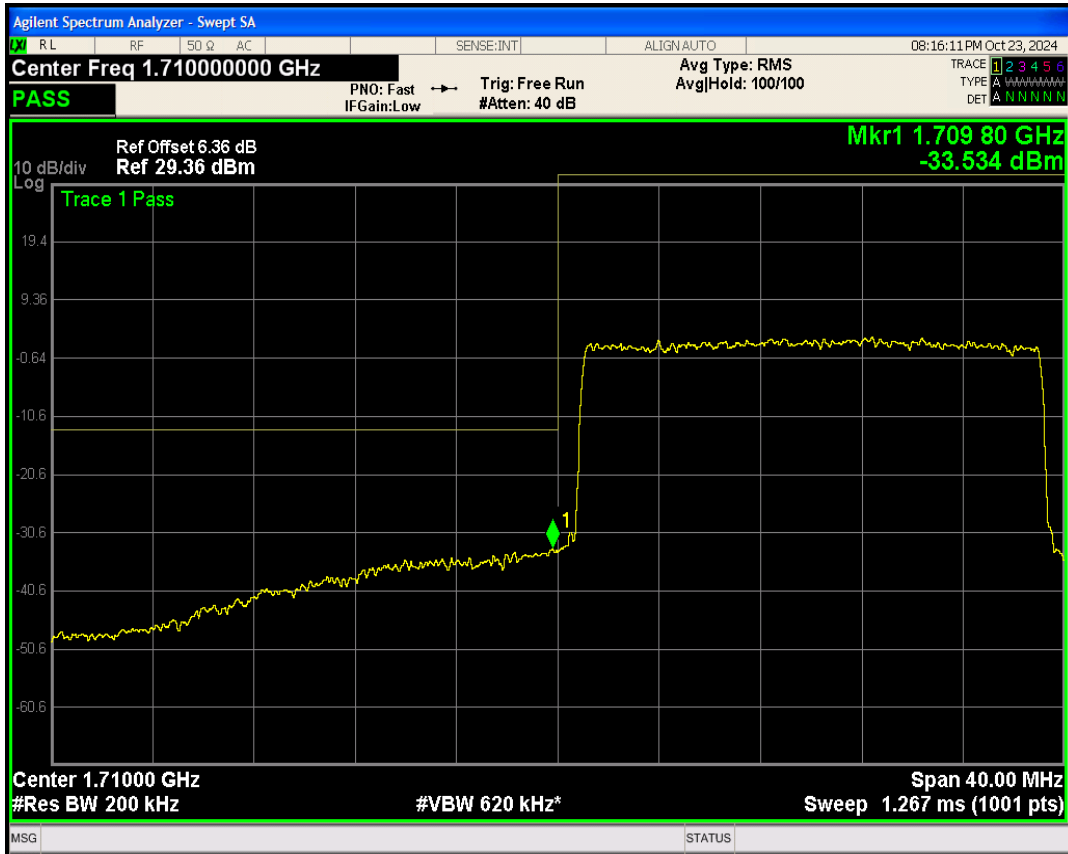
Band4 QPSK BW=20MHz Channel=20300 RB Size=100 Position=#0
