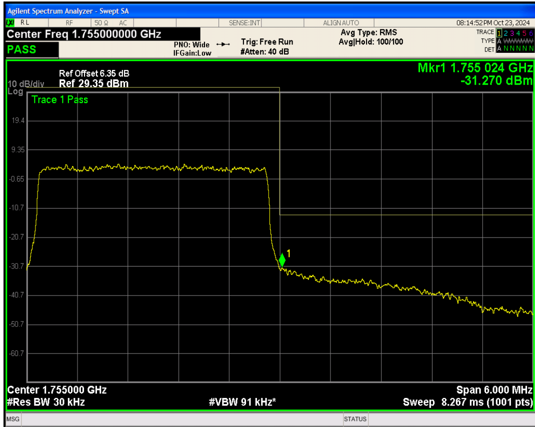
Band4 16QAM BW=3MHz Channel=20385 RB Size=15 Position=#0
