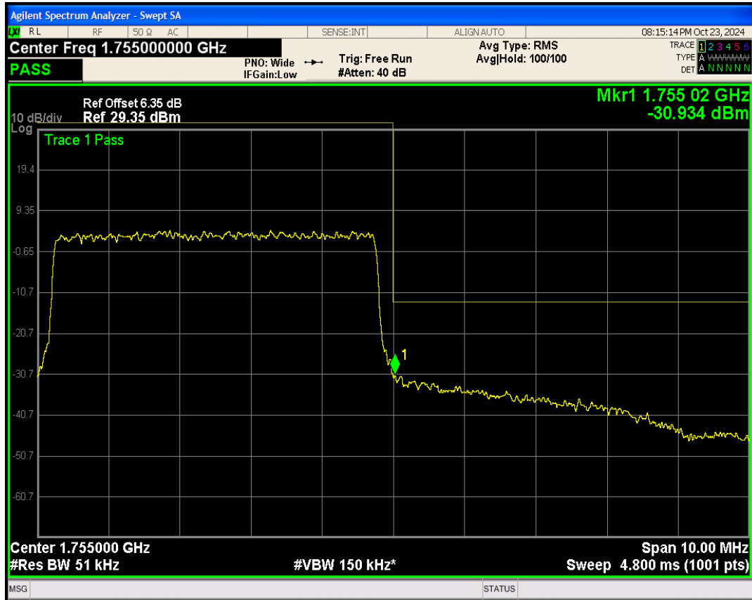
Band4 16QAM BW=5MHz Channel=20375 RB Size=25 Position=#0
