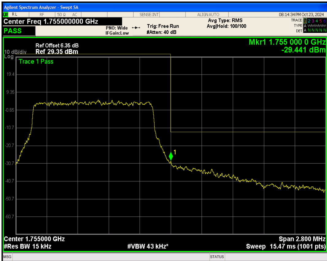
Band4 QPSK BW=3MHz Channel=19965 RB Size=15 Position=#0
