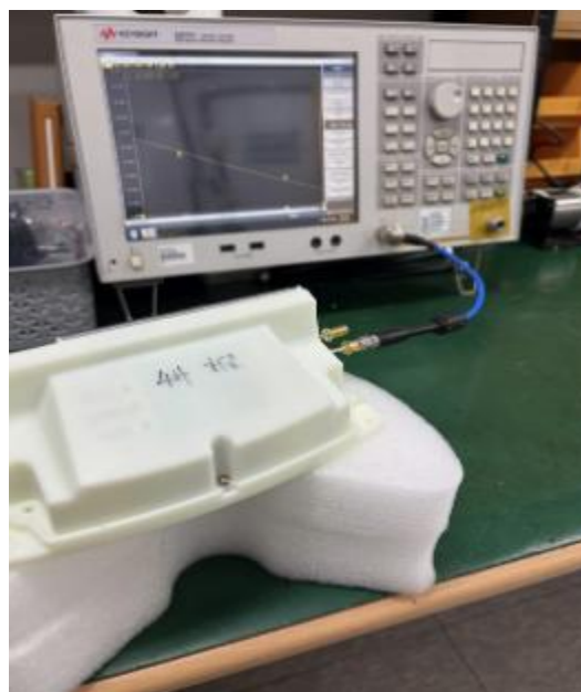
Figure 1. (Network Analyzer) Electrical Characteristic Measurement
