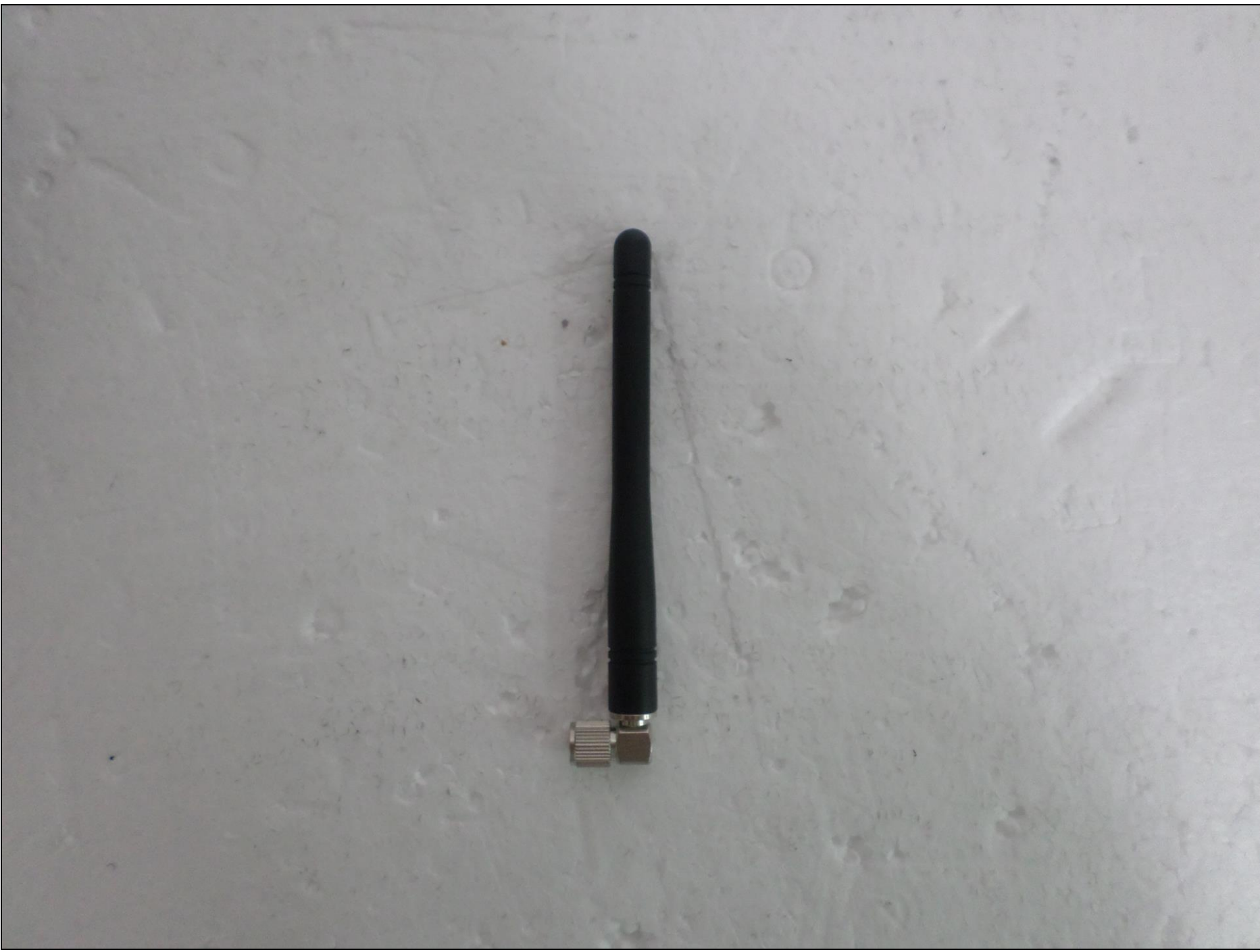
View of LTE Antenna
