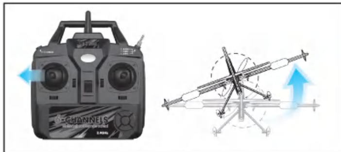
(5).左倾斜：将遥控器左操纵杆向左移动时，飞机随之向左倾斜。 Left tilt: When the left joystick of the remote control is moved to the left, the aircraft will tilt to the left accordingly.
