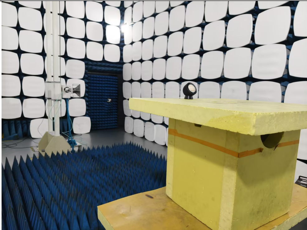
Radiated Spurious Emission, Above 1GHz
