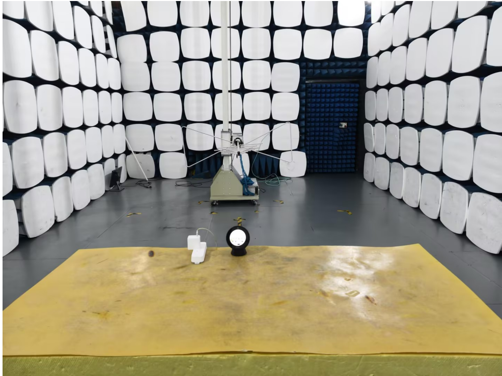
Radiated Spurious Emission, Above 1GHz
