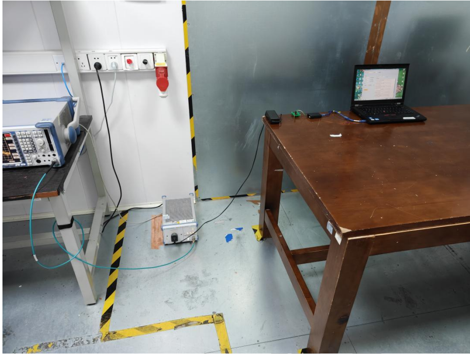
Conducted emissions at AC power line (150kHz-30MHz)
