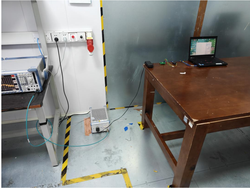
Conducted emissions at AC power line (150kHz-30MHz)
