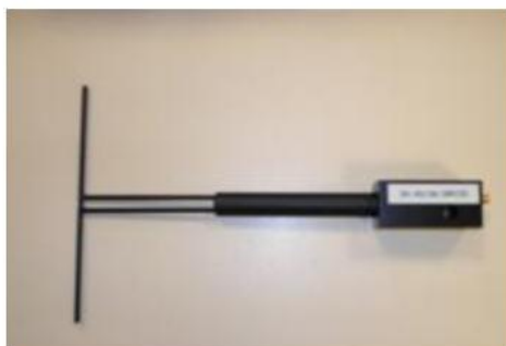
Figure 1 – Satimo COMOSAR Validation Dipole
