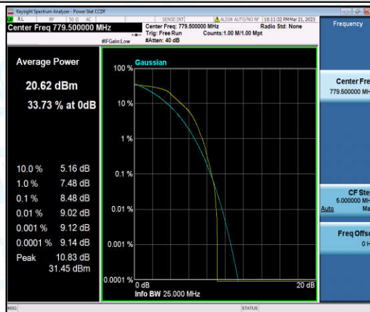
Band13-5MHz-16QAM-23205-6-0-Low-8.48-<=13-PASS
