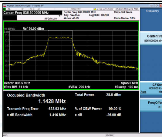
Band26-3MHz-QPSK-26915-6-0-Low-1.1428-1.416-PASS
