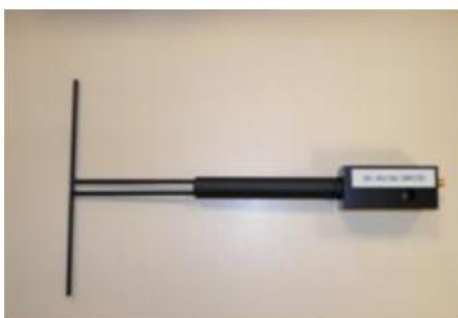
Figure 1 – Satimo COMOSAR Validation Dipole
