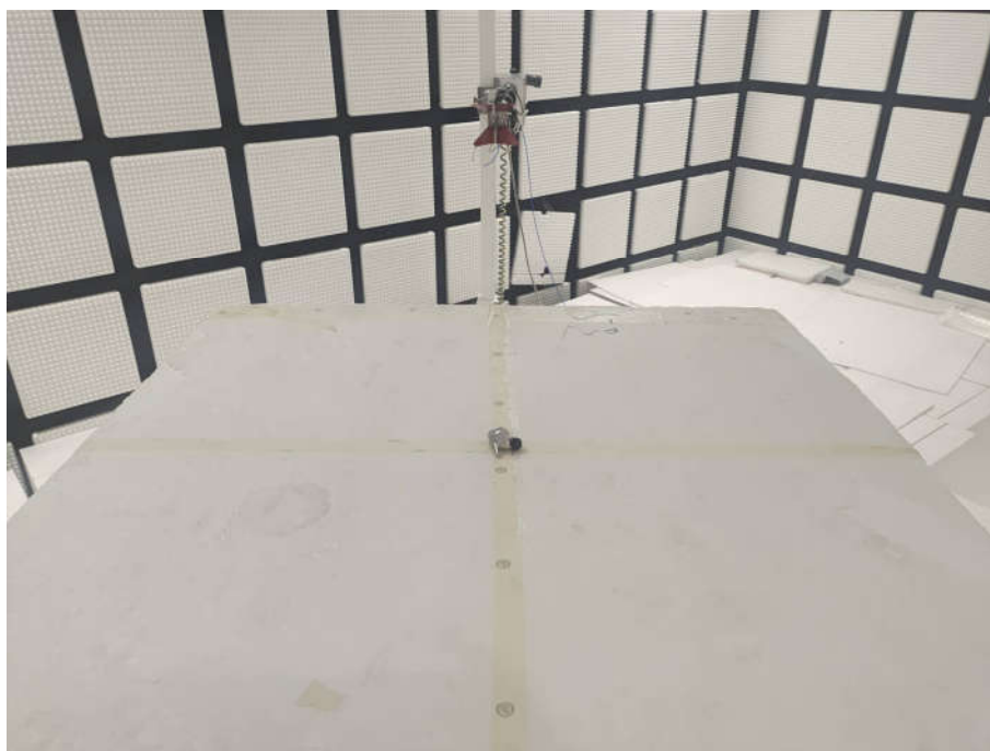
Radiated spurious emission Test Setup-3(Above 1GHz)
