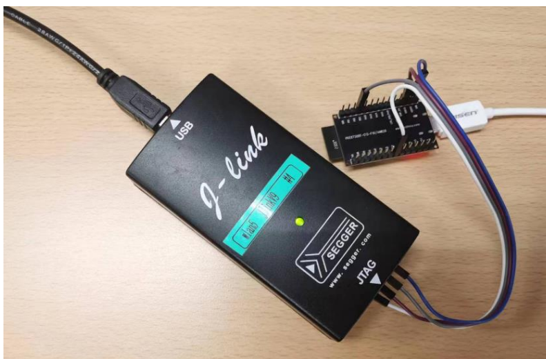
Fig 1-3 J-Link and Ameba-D SWD connection
