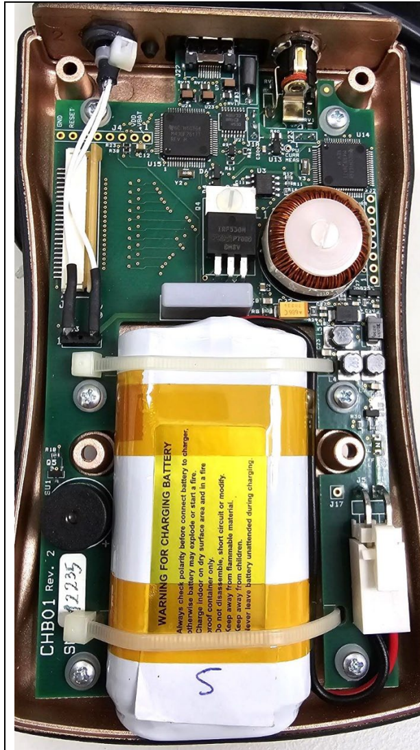
Battery Charger Internal Photo, Front of PCBA
