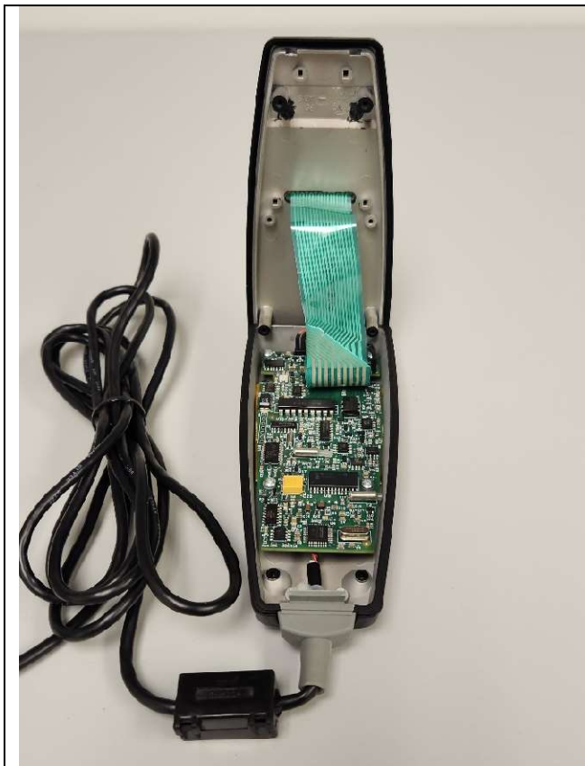
Programmer Wand Internal Photo, Case Disassembled
